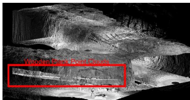
Figure 1.9 - Planks Merged with Tunnel
