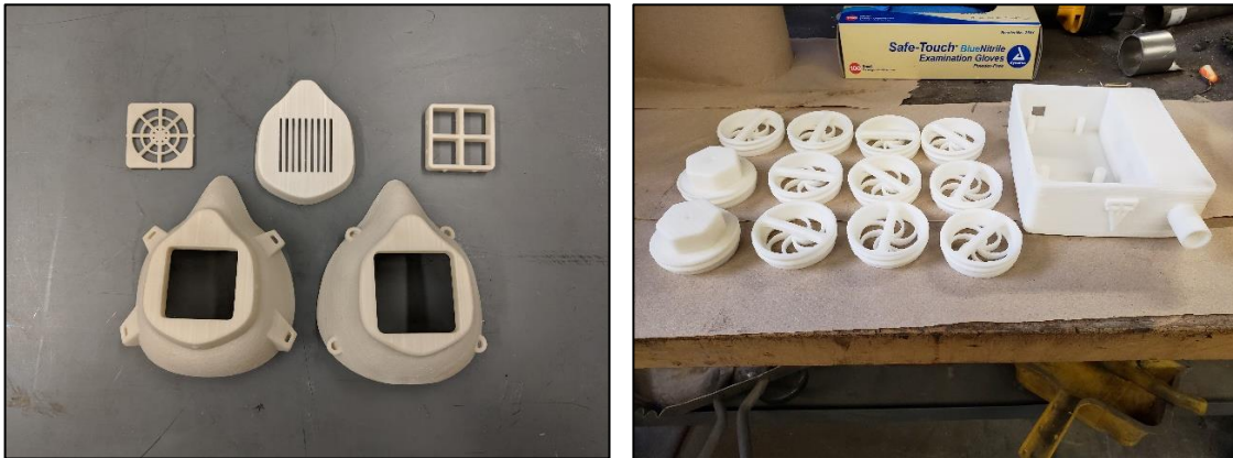
Figure 6 – Face mask (left) and respirator components surface finished at Ware Lab for VT Carilion in Roanoke.
