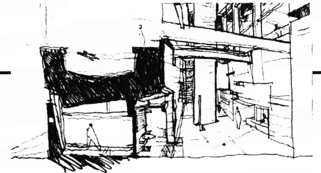
Section model of one bay of the 103rd street side of the project showing the shear walls containing the low income dwellings; with the edge screen along the street and the porches, stoops and galleries along the courtyard edge. The pool and bath slide under the dwellings and the basketball court and handball courts push under the courtyard
