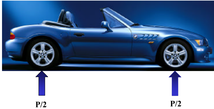
Figure 31. Vehicle loading for car (or truck/SUV). The load of the vehicle is assumed to be evenly divided among the axles.
