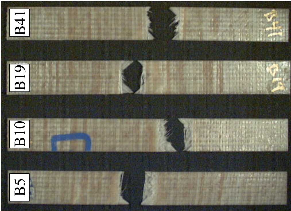
Figure 36. Failed specimens for the High-Low condition. Note that the specimens show little fiber pullout.
