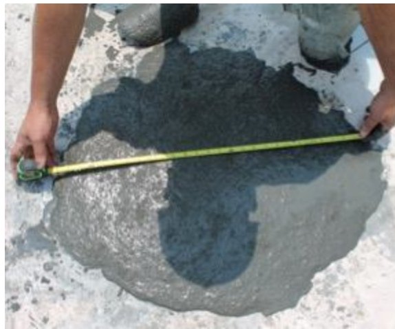
Figure 125. Slump test, VHPC too flowable
