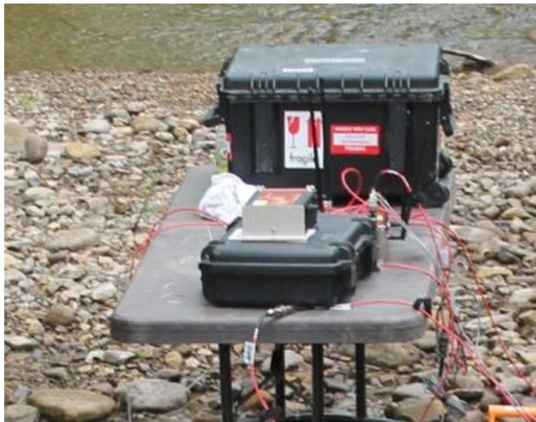
Figure 44. DAS base station
