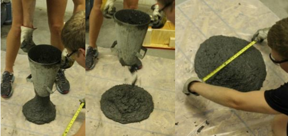
Figure 27. Inverted Cone and Slump Testing
