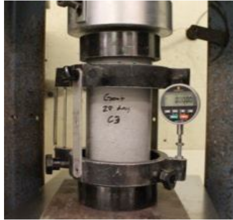
Figure 18. Modulus of Elasticity Test
