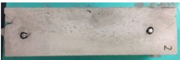
Figure 33. Shrinkage bar with discs and DEMEC extensometer
