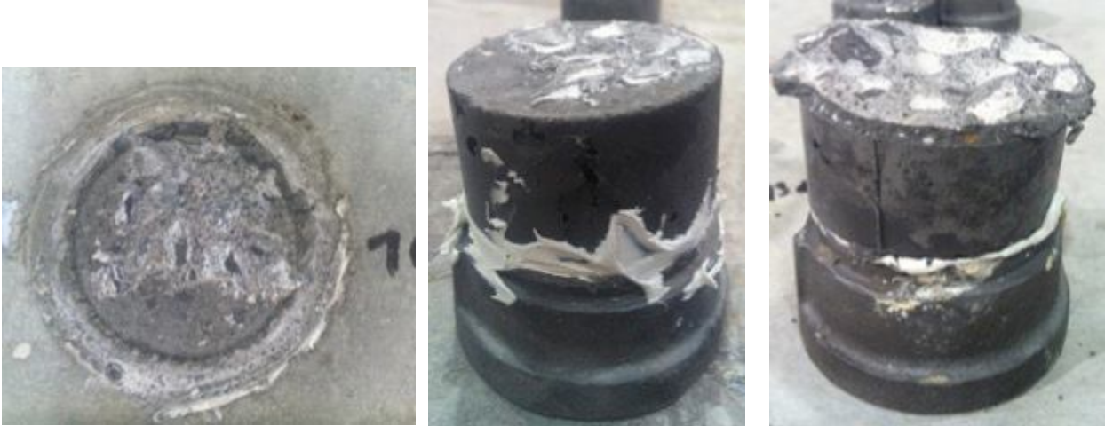
Figure 78. Typical VHPC 7 days and older failure
