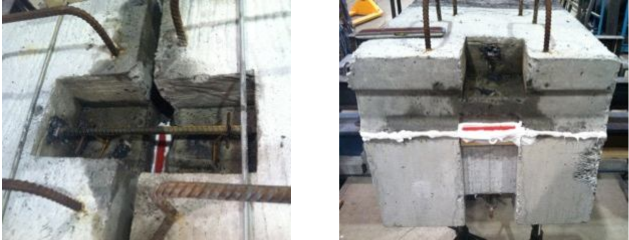
Figure 35. Non-contact voided slab connection
