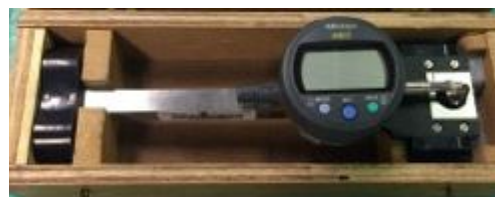
Figure 33. Shrinkage bar with discs and DEMEC extensometer
