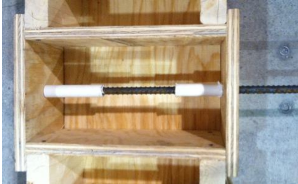
Figure 20. Bonded vs debonded reinforcing steel for pull out specimen
