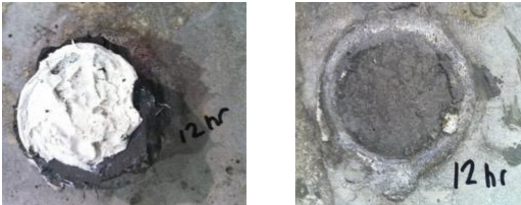
Figure 76. Typical VHPC 12 hour to 1 day failure
