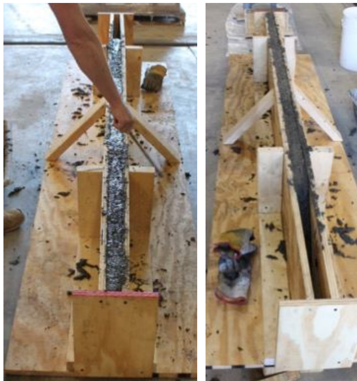
Figure 29. Shear key flow test
