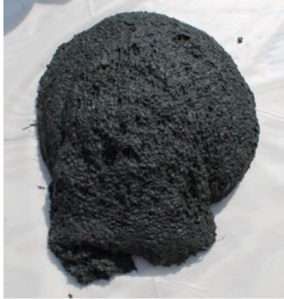
Figure 124. Slump test, VHPC too stiff
