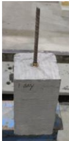
Figure 69. Ruptured reinforcing steel
