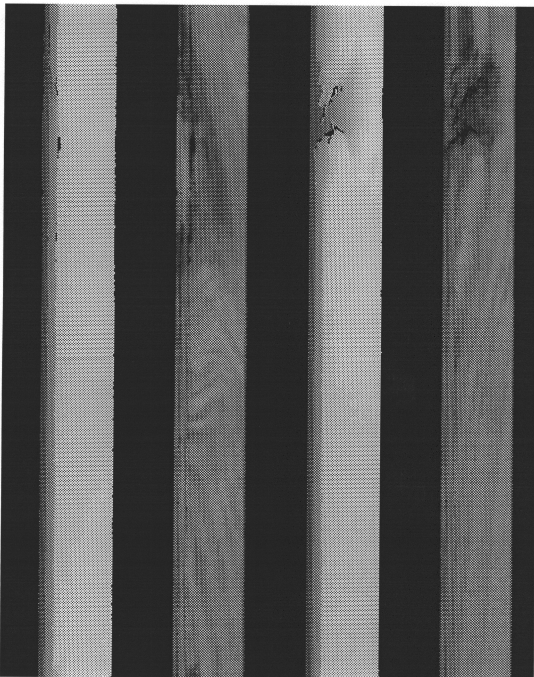
Figure 7.6 From left to right: (A) range in registration with (B) intensity, (C) and (D) are continuous parts of (A) and (B). These registration pair images are generated by the Range and Total-Reflectance Processors.
