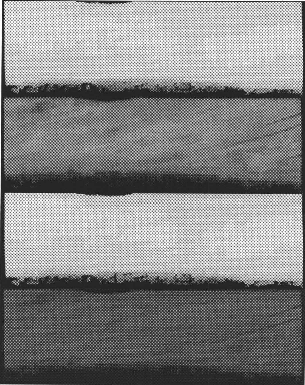
Figure 7.10 Comparisons of registered image pairs. From top to bottom: (A) range in registration with (B) intensity (Total-Reflectance), (C) range in registration with (D) intensity (Center-Pixel Intensity). Board E.
