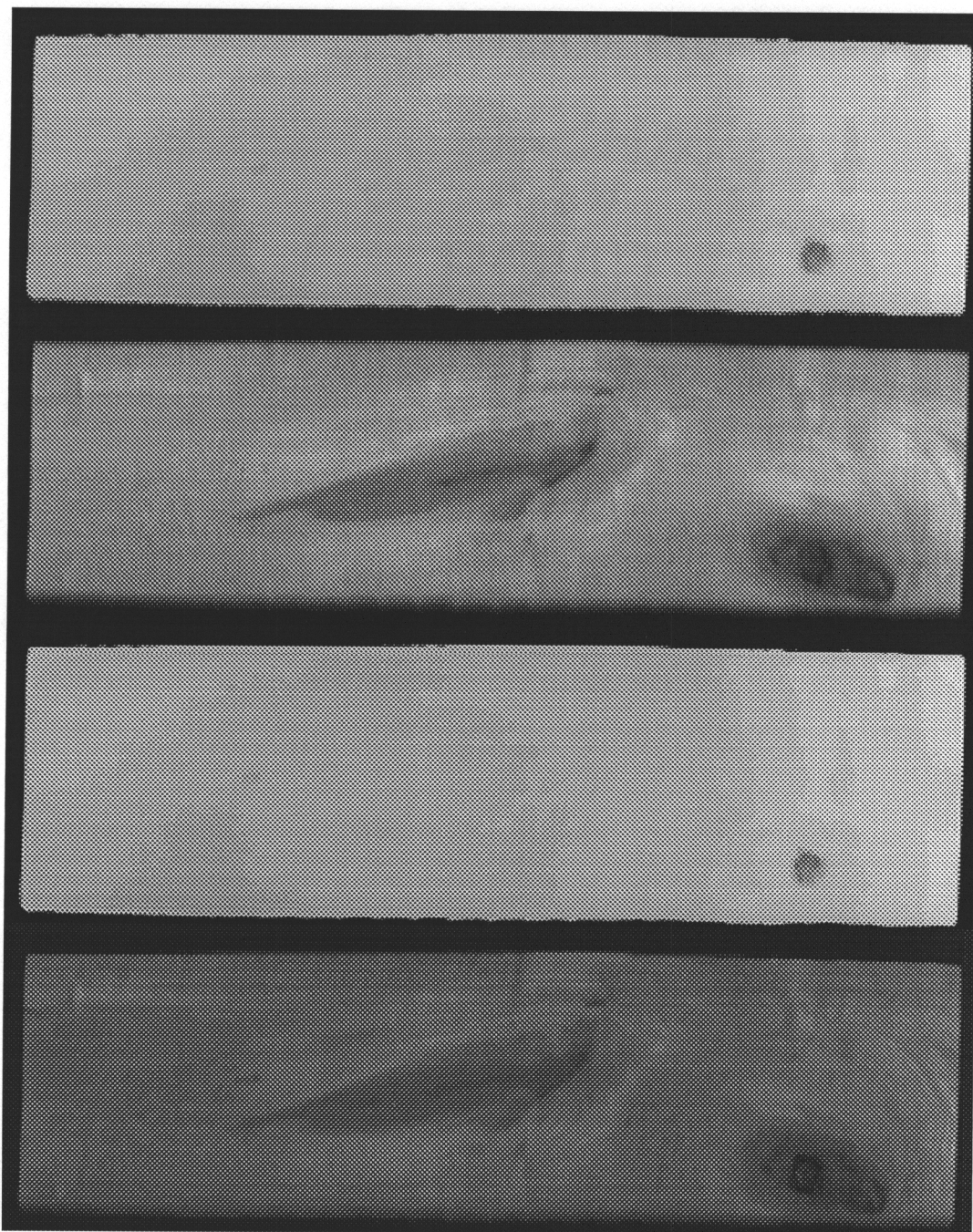
Figure 7.7 Comparisons of registered image pairs. From top to bottom: (A) range in registration with (B) intensity (Total-Reflectance), (C) range in registration with (D) intensity (Center-Pixel Intensity). Board B.
