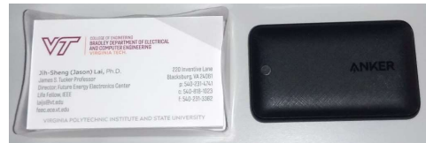
GaN device based universal charger, size: smaller than a business card, 56 g
