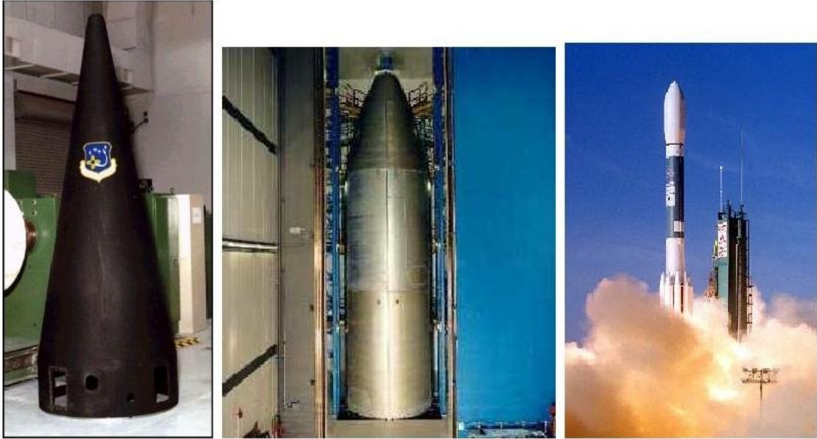
Figure 1.1: Various shroud geometries: a.) grid stiffened USAF launch vehicle payload fairing, b.) Titan IV payload fairing by Lockheed Martin and c.) Delta II payload fairing by Boeing during launch.
