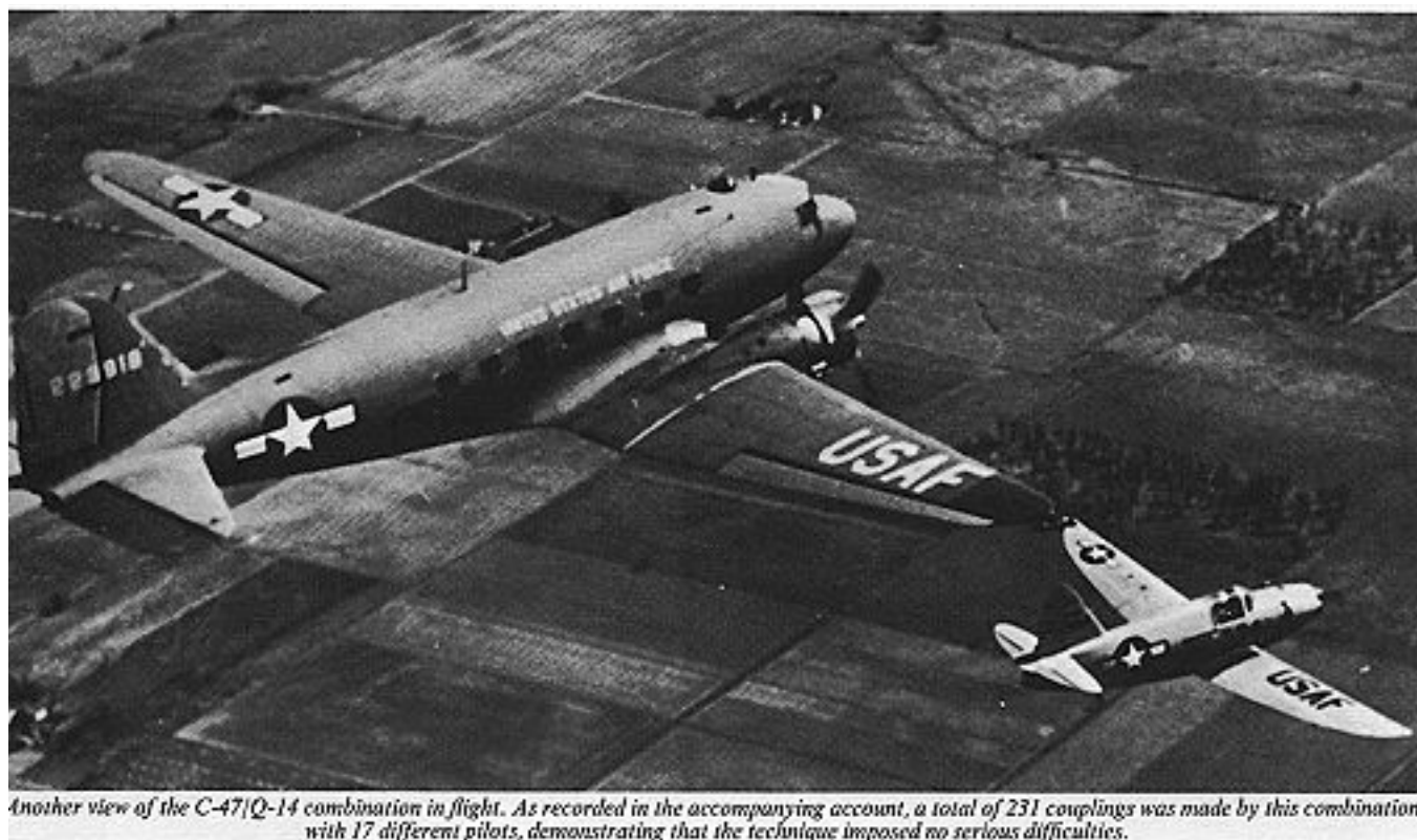
Figure 1.9: Aerial Photograph of C-47/Q-14 Wingtip Docking Flight Tests[1]
