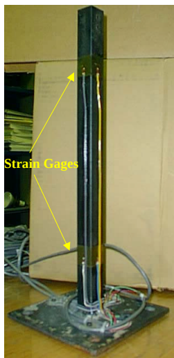
Figure 2.7: Four Component Strut Balance to Measure Forces and Moments on the Transport Wing Model
