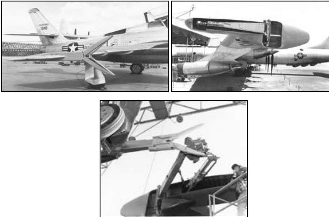
Figure 1.12: (Top left) The Jaw Mechanism on the F-84, (Top right) the Pod Appendage on the B-36 Wing, (Bottom) the Engagement Mechanism for Tom Tom Clamping onto the Articulated Arm Extending from the Pod Appendage [2].
