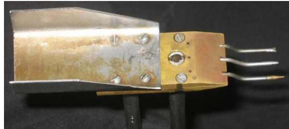
Figure 4.3: Aero-Thermodynamic triple rake probe (top) Pitot Probe (middle) Total Temperature Probe (bottom) Cone-Static Probe
