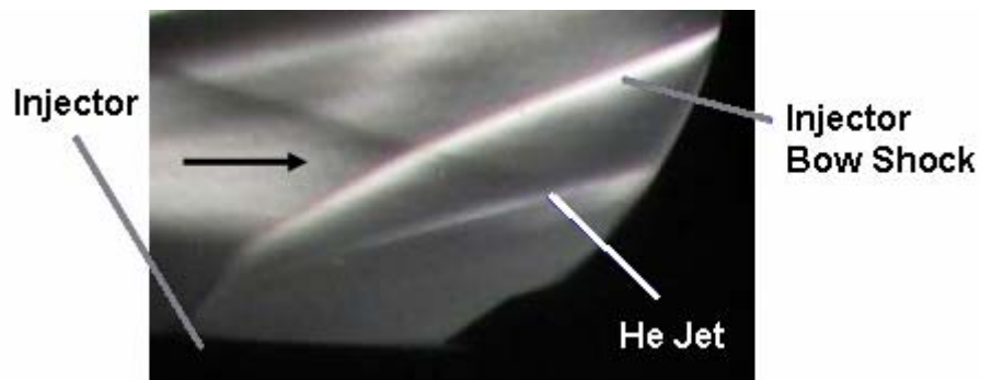
Figure 3.2: Schlieren photograph of helium injector in crossflow
