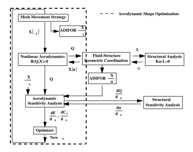
Figure 1.2: Aerodynamic shape sensitivity analysis and design optimization.
