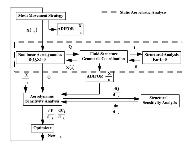
Figure 1.3: Static aeroelastic analysis.
