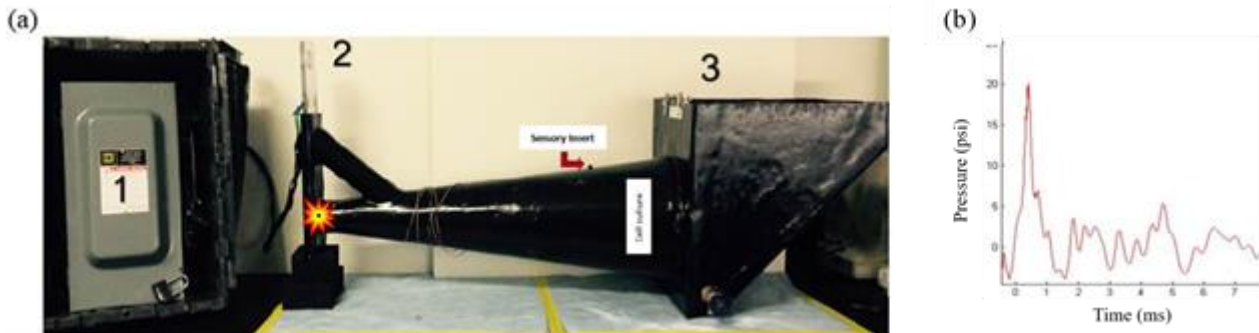
Figure 3.2 High-Rate Overpressure Simulator - In Vitro Injury Model of bTBI. (a) The HOS is a water-filled chamber that exposes in vitro samples to high-rate overpressure via an exploding bridge wire mechanism. 1) Driver for the energy required (high electrical current); 2) Bridge wire mechanism (wire holder), and 3) Cell culture plate location and sensory insert. Upon wire vaporization, the wave front travels down the test section of the cell culture plate denoted by “Cell Culture.” (b) Pressure profile: The high-rate compression waves, as represented in the pressure profile, is meant to mimic an intracranial high-rate overpressure.
