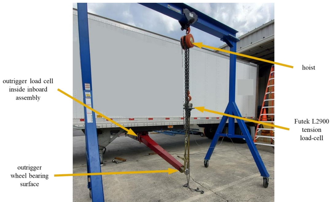
Figure 5-8. Test setup for determining the force ratio from the outrigger wheel to the outrigger load cell.
