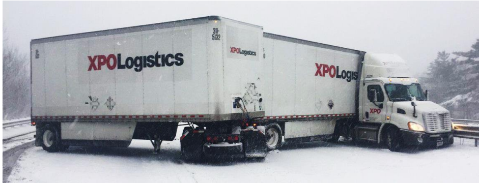
Figure 2-12. Jackknifed A-train double (Massachusetts State Police, 2019).
