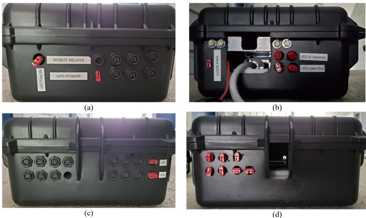
Figure 5-11. Junction box external connections. (a) Tractor sensor connectors and GPS power. (b) Tractor DB-37 output and DB-37 input from front trailer, LiDAR power port and connectors for flag LEDs on the tractor. (c) Trailer analog sensor connectors and power ports. (d) Trailer flag LED connectors and cutout for DB-37.
