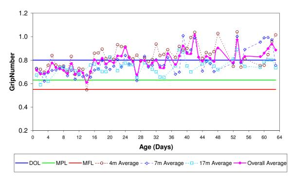
Figure 7 – The Lowest Minimum 100m Rolling Average Friction at 4m, 7m and 17m Offsets [11]
