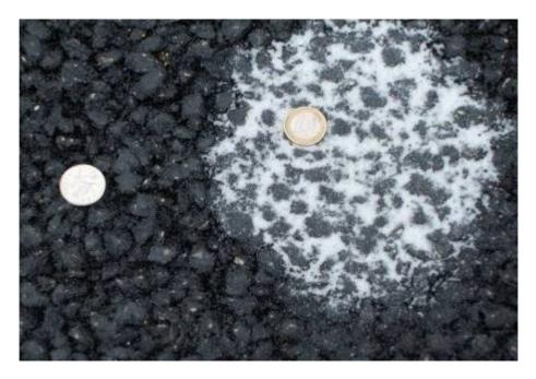
Figure 1 – A Typical Surface Texture of Ungrooved AC-14 BBA D
