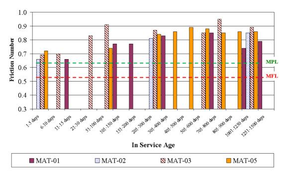
Figure 3 - In Service Friction Values for Grooved BBA
