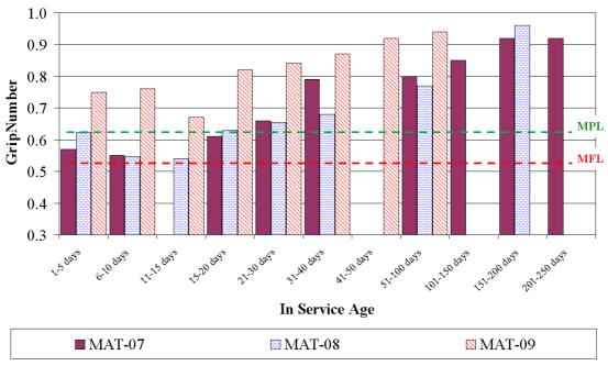
Figure 5 - In Service Friction Values for All BBA (ungrooved) to Date
