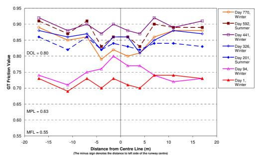
Figure 2 – Changes in Friction Value with time, measured by Grip Tester, at 0.25mm water depth
