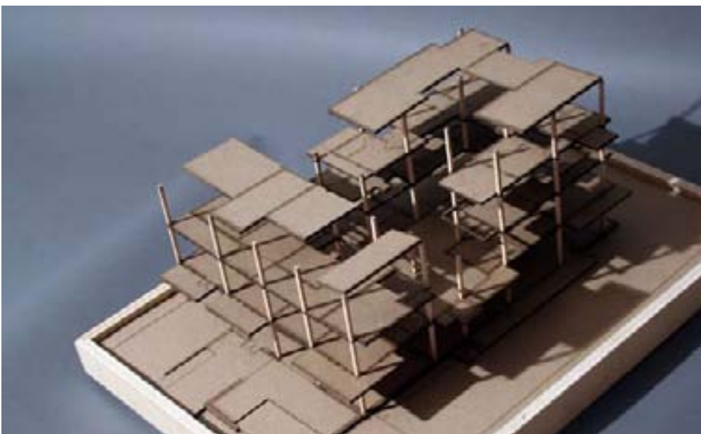
MASSING MODEL EXPLORING CONCRETE COLUMN AND FLOOR SLAB STRUCTURE. (FINAL ITERATION)
