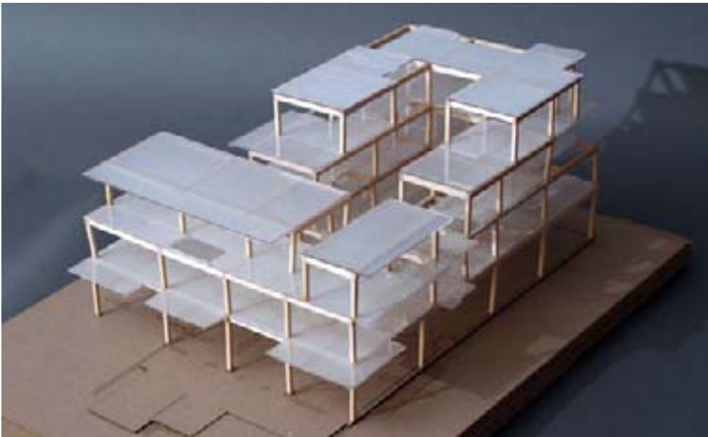
MASSING MODEL EXPLORING COLUMN AND FRAME STRUCTURE
