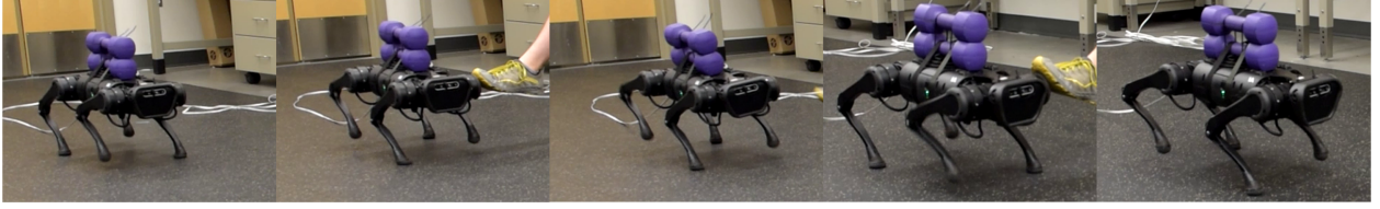
Figure 2.2: This experiment displays A1 trotting under the influence of both a 4.54 (kg) payload (36% of the robot’s weight) and push disturbances. The quadruped was able to resist these uncertainties and continue trotting. Videos of the experiments are available online [9].
