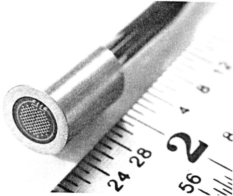
Figure 2.1.5 The HFM-6 Heat Flux Microsensor mounted in an aluminum housing and equivalent to the insert gages used on the pressure side (dimensions in inches).
