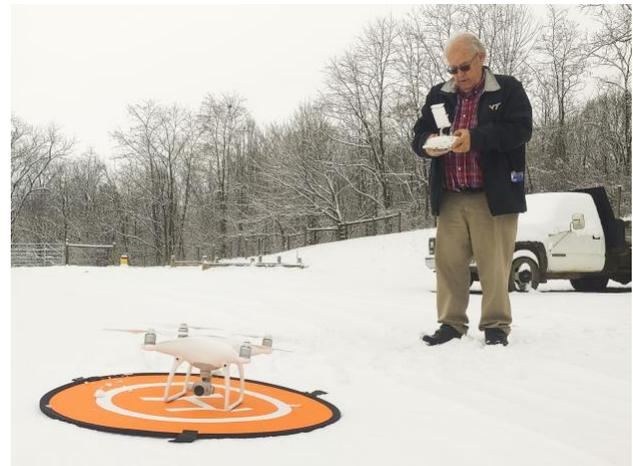
Figure 1: Using a landing pad like the one pictured reduces the drone's contact with moisture during takeoffs and landings.
