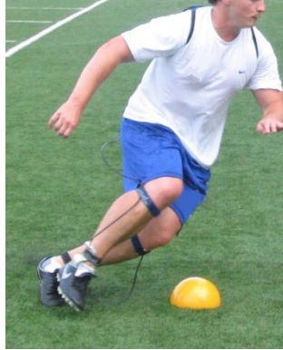
Figure 1: pedar® In-shoe Pressure Distribution Measurement with Backpack
