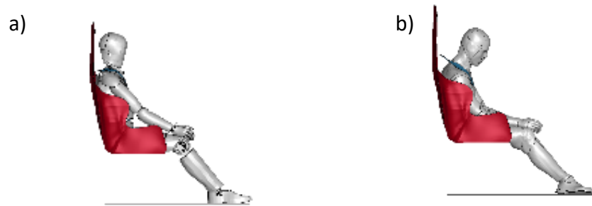
Figure 24 Occupant position at peak HIC value for the 42g rigid seat test condition a) THOR, b) GHBMC Standard Position
