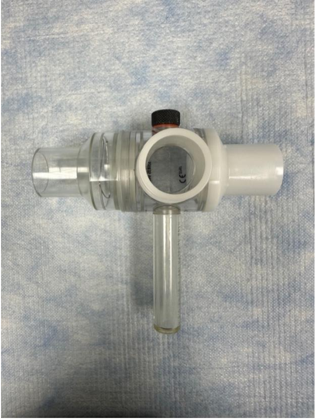
Image 1. Mouthpiece set-up for air collection during jumping exercises.
