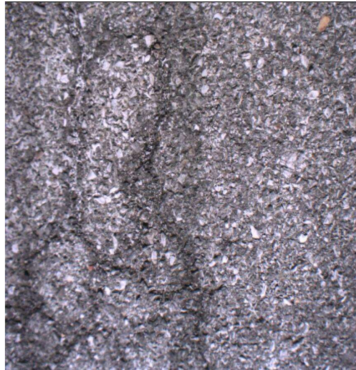
(a) An image of the flat plate stuck with mimic road pattern.
