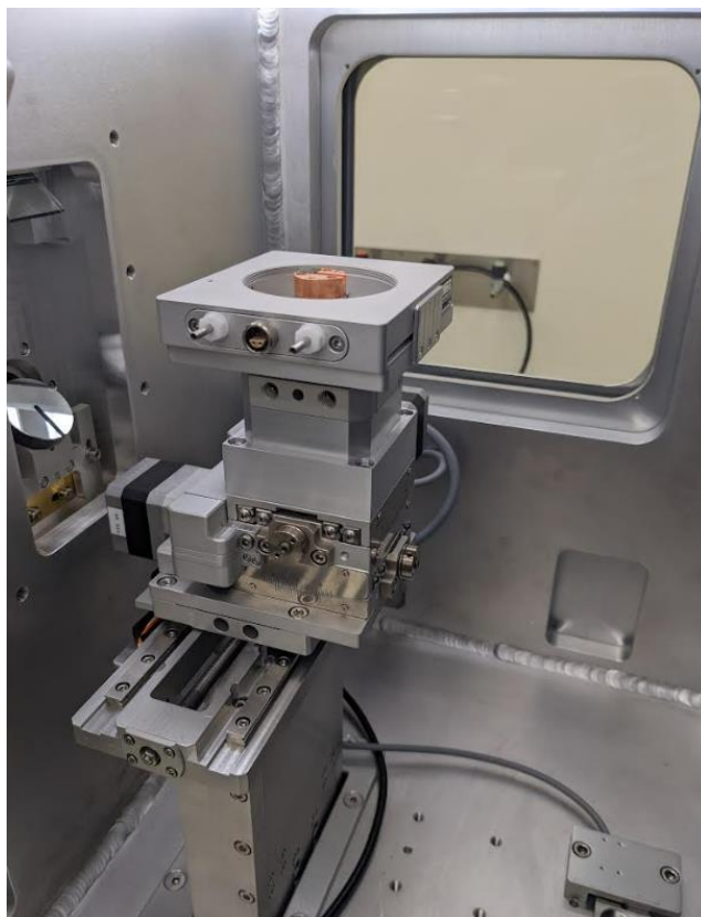
Figure 7.36. Photograph of the Linkam temperature stage attached to the grazing incidence stage on the Xenocs Xeuss 3.0 SAXS/WAXS system at Virginia Tech.
