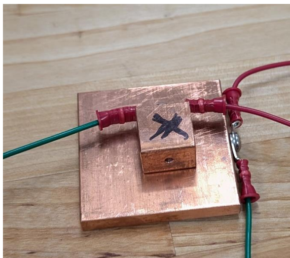
Figure 5.12. A custom copper testing geometry designed and manufactured by Scribner, LLC for testing the gross electrical shortage of MEAs prior to fuel cell testing. The MEA is placed in the center of the setup, with copper blocks underneath and on top of the MEA, creating a sandwich. The leads are connected to a potentiostat.
