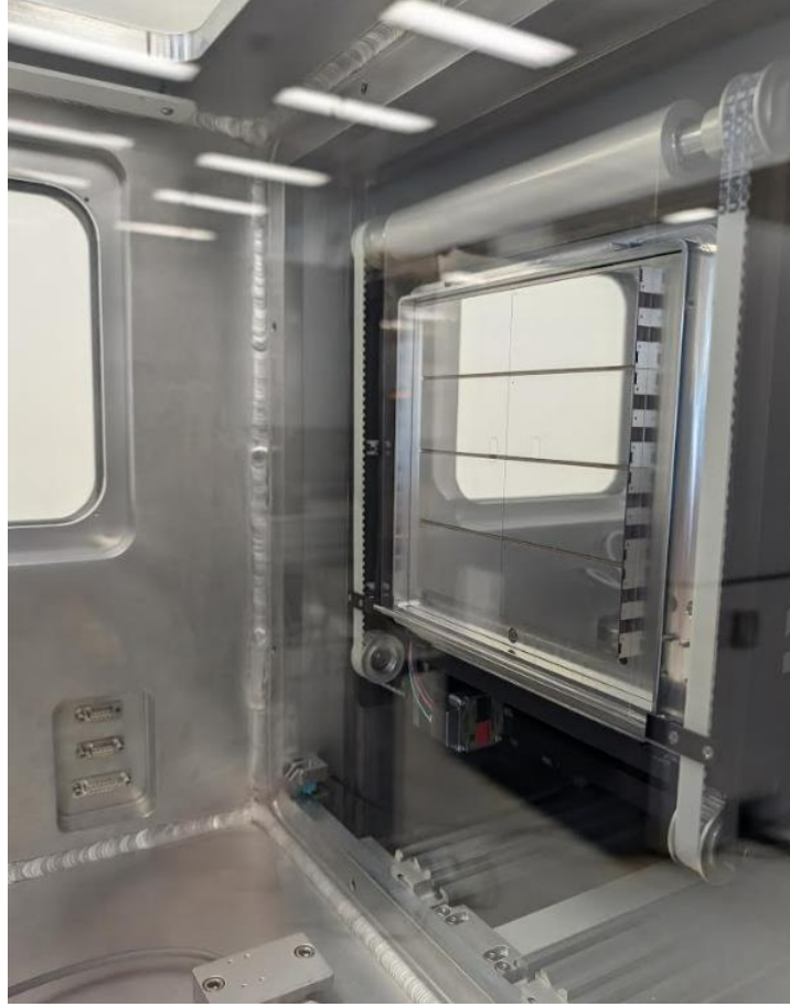
Figure 2.11. Dectris Eiger2 4M detector on the Xenocs Xeuss 3.0 SAXS/WAXS system. A protective plastic film covers the detector during changes in pressure, including chamber evacuation and venting.
