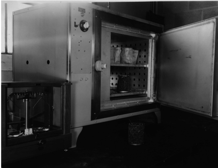
Fig. (4). Forced draft oven, analytical balances, and wire mesh containers.
