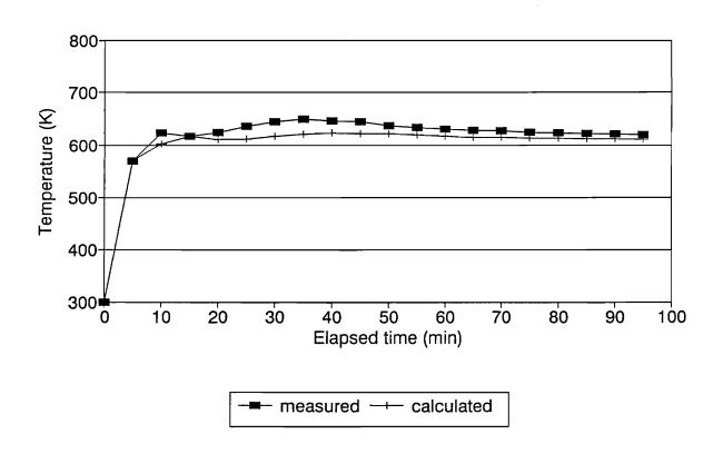
Figure 21. Comparison of measured and predicted temperatures. Results for the interior surface of the contraflow's wall.
