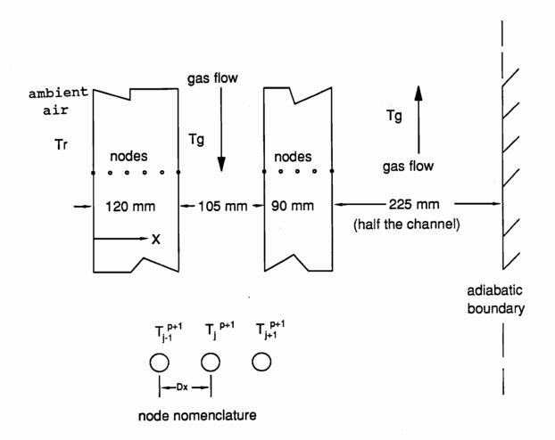
Figure 1. Finite Difference Model of the Contraflow Heat Exchanger in the TU2500L
