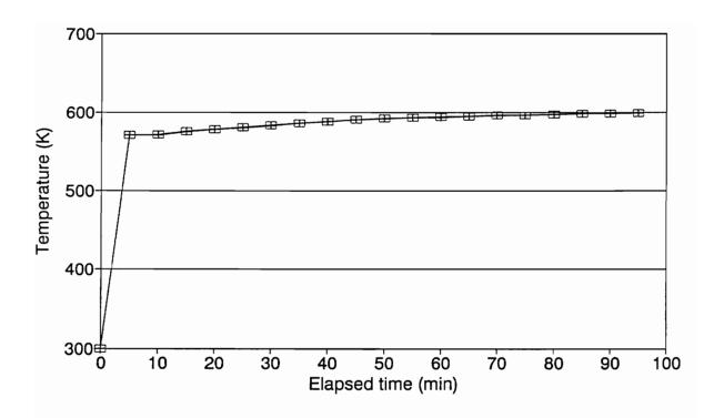
Figure 18. Check on the assumption of symmetry about the heater's centerline. Results for two symmetrically placed thermocouples in the contraflow. Data shown by open square and plus symbols.
