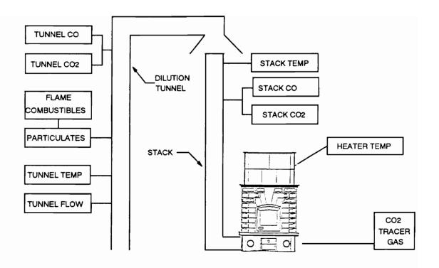
Figure 2. Stack and Tunnel Sampling System
