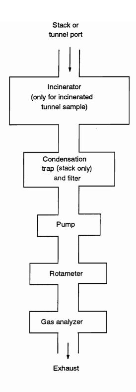
Figure 3. Gas Sampling Flowchart
