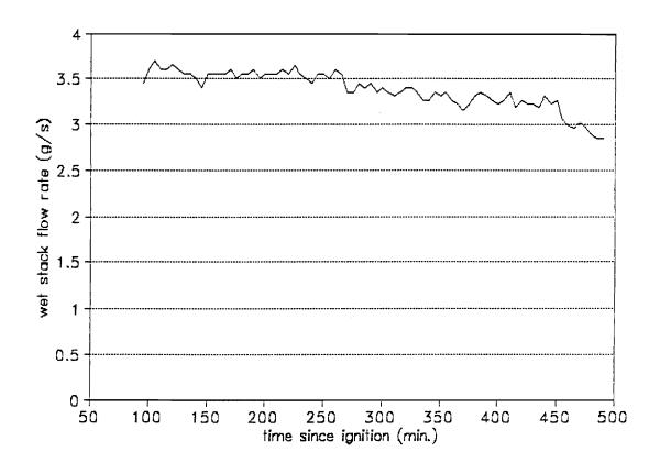
Figure 15. Typical stack flow rates during the off-period.
