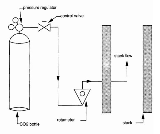
Figure 6. Tracer Gas System
