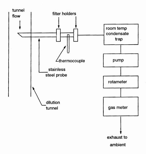
Figure 4. Particulate Matter Train Setup
