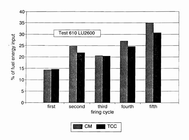
Figure 9. Comparison of on-period sensible energy losses using the TCC and CM methods. Results for one test with the bake oven.
