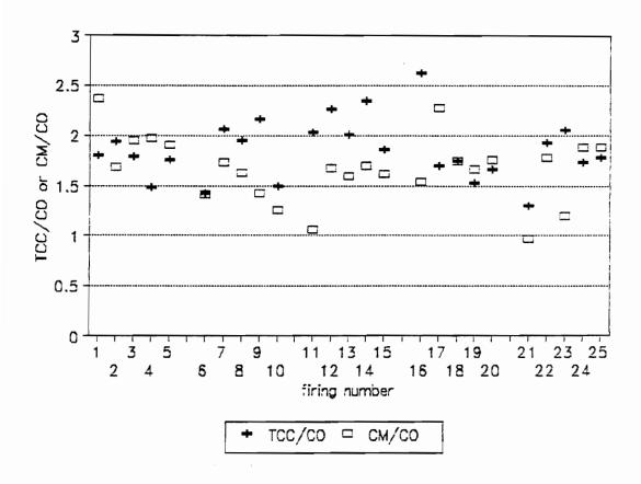
Figure 11. Ratio of total chemical energy losses to the chemical loss due to CO. Results for Tests 605, 606, 607, 610, and 611.
