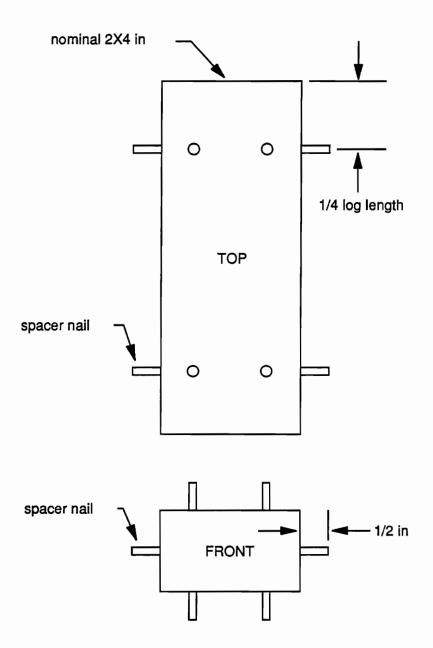
Figure 8. Main Load Fuel Piece
