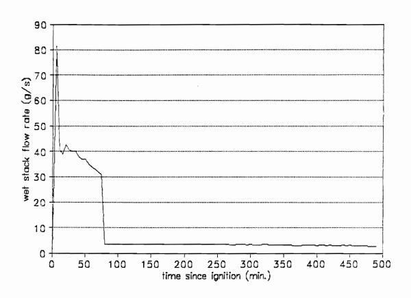
Figure 16. Stack flow rates during the on and off periods.
