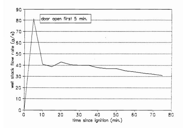
Figure 14. Typical masonry heater stack flow rates during the on-period. Results for one firing with the contraflow
