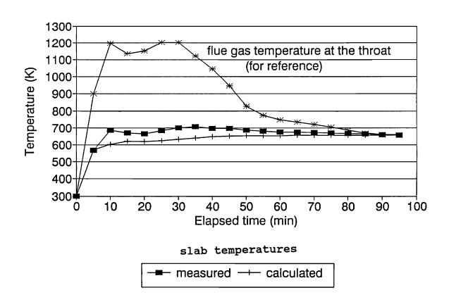
Figure 20. Comparison of measured and predicted temperatures. Results for the left surface of the contraflow's internal slab.
