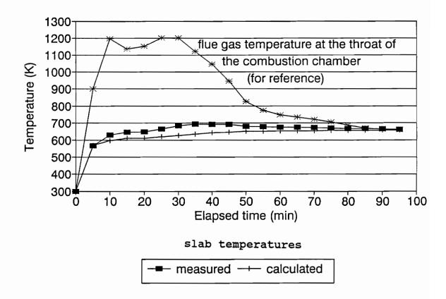
Figure 19. Comparison of measured and predicted temperatures. Results for the right surface of the contraflow's internal slab.
