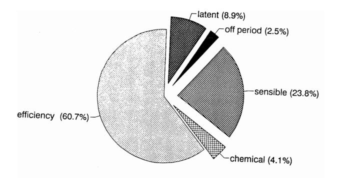
Figure 13. Distribution of energy losses for the fifth firing of one test with the contraflow.
