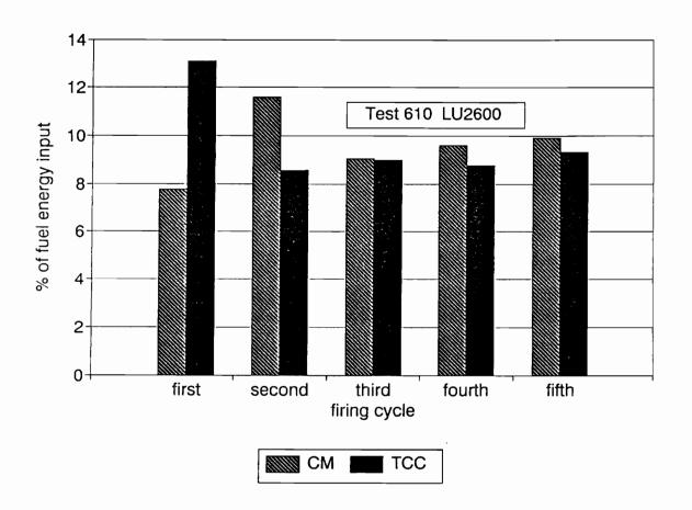
Figure 10. Comparison of chemical energy losses using the TCC and CM methods. Results for one test with the bake oven.
