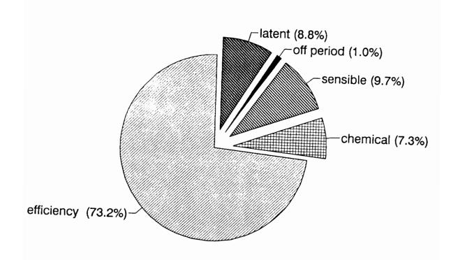
Figure 12. Distribution of energy losses for the first firing of one test with the contraflow heater.
