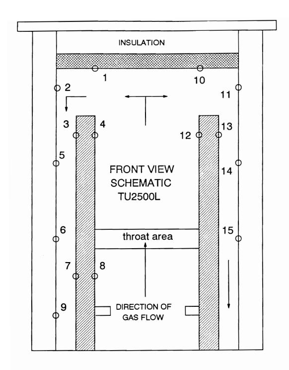
Figure 7. Thermocouple Placement in the contraflow masonry heater
