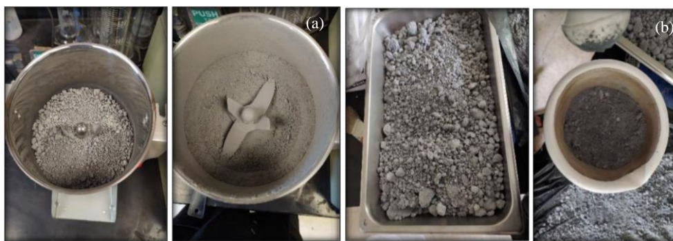
Figure 15. Comminution process (a) BA sample pulverized in an electric mill, b) FA non-mechanical comminution.
