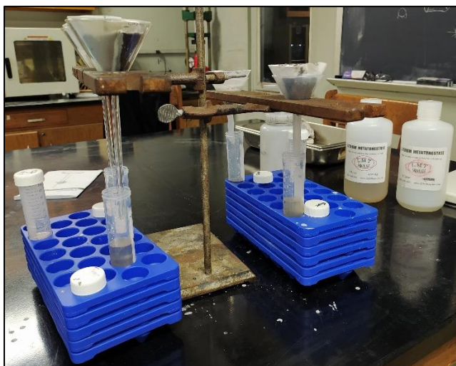
Figure 16. Float- Sink test set up.
