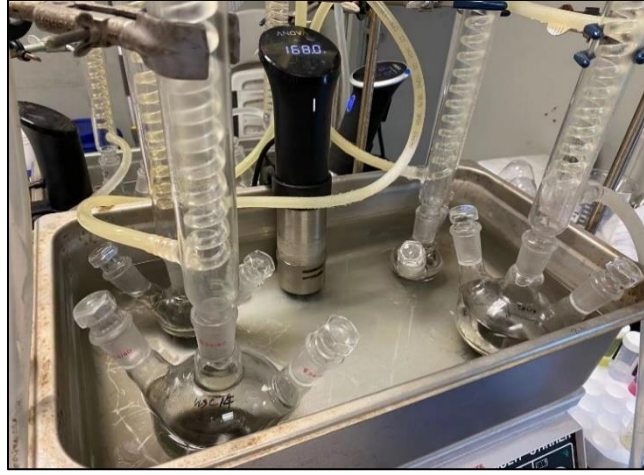
Figure 19. Experimental set up used for the acid leaching tests.
