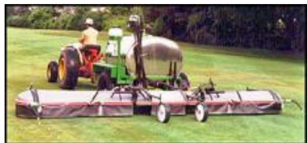
Figure 11. Shield booms minimize the effect of wind on the spray pattern and thereby reducing drift potential.
