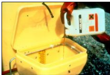
Figure 10. Chemical inductor for a sprayer to reduce operator exposure to pesticides and to clean empty chemical containers.
