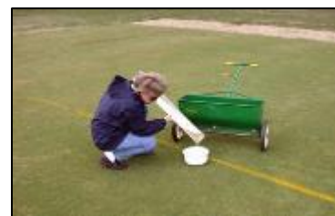
Figure 25. Attach a calibration pan beneath the spreader so that when the spreader is pushed over the calibration course, the output is collected.
