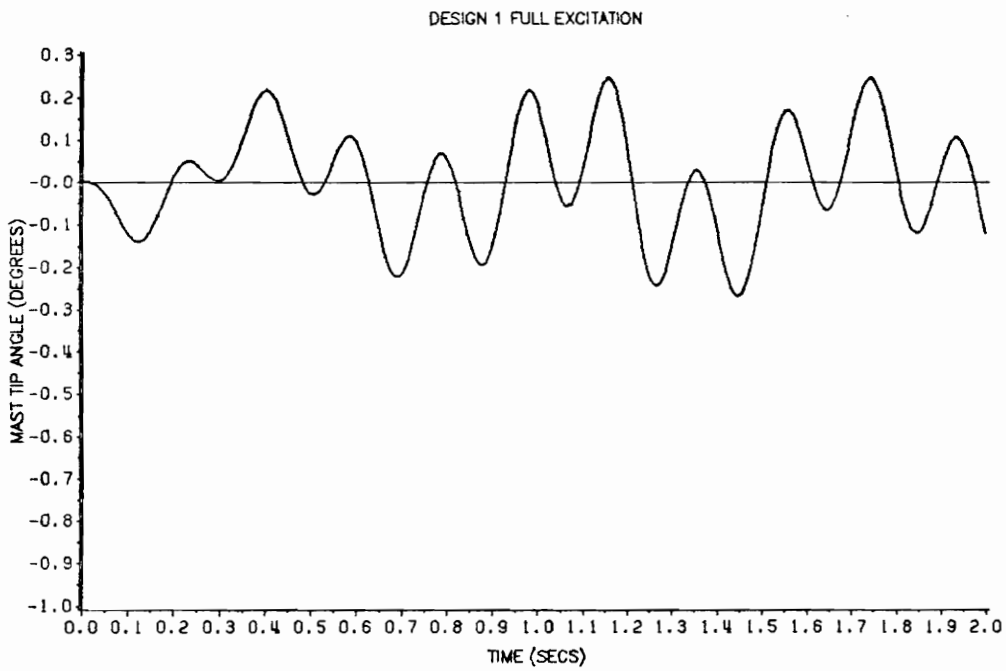
Figure 29. Simulations of Mast Tip Angle, Design One.: Top, \delta_{c,2,4} = \pm 100.0 \sin 9.11t
