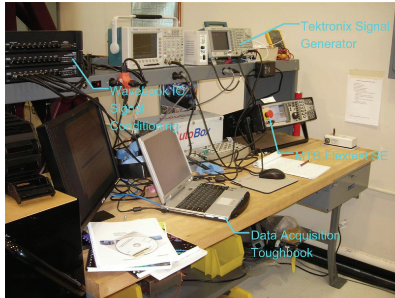
Figure 5-6. Data acquisition and instrumentation for actuator control and collection of data.
