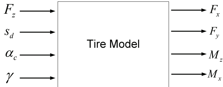
Figure 4-10. Minimum inputs/outputs to and from a tire model for vehicle dynamics simulation
