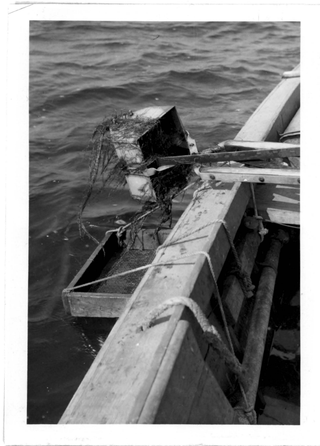
Figure 10. Bottom Sampler and Sieve in Use.
