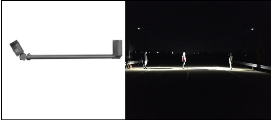
Figure 5. Photo. Saalex LED floodlight CWI and resulting illumination of pedestrians in the crosswalk when used alone.
