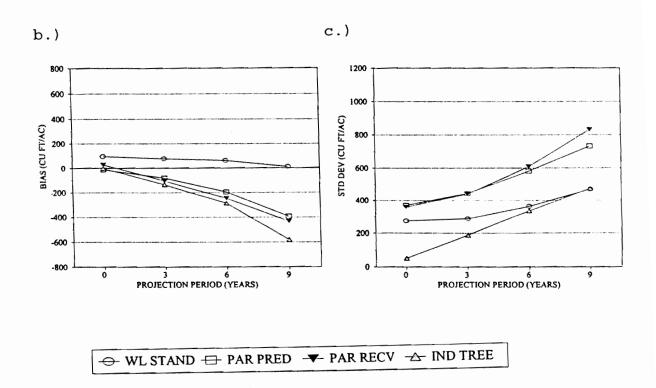
Figure 3. Graphed Results from 50/50 Double Cross Validation by model type for set 1: a.) RMSE versus Projection Period, b.) Bias versus Projection Period, c.) Standard Deviation versus Projection Period
