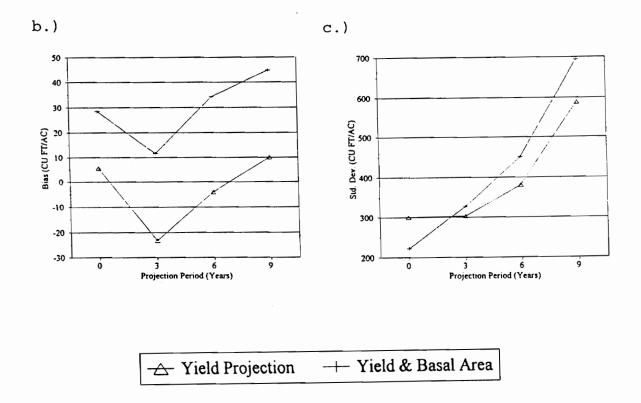
Figure 6. Graphed Results from Whole Stand Yield Analysis by Parameter Estimation Procedure: a.) RMSE versus Projection Period, b.) Bias versus Projection Period, c.) Standard Deviation versus Projection Period
