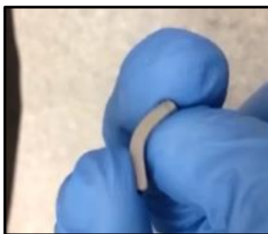
Figure 5 Polyurethane in 1-butanol, bending
