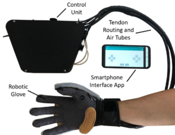
Figure 2.10: Hybrid Exoskeleton Glove with a Telescopic Thumb [11]
