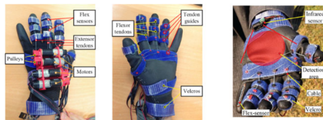
Figure 2.6: Portable Exoskeleton Glove With Soft Structure [7]
