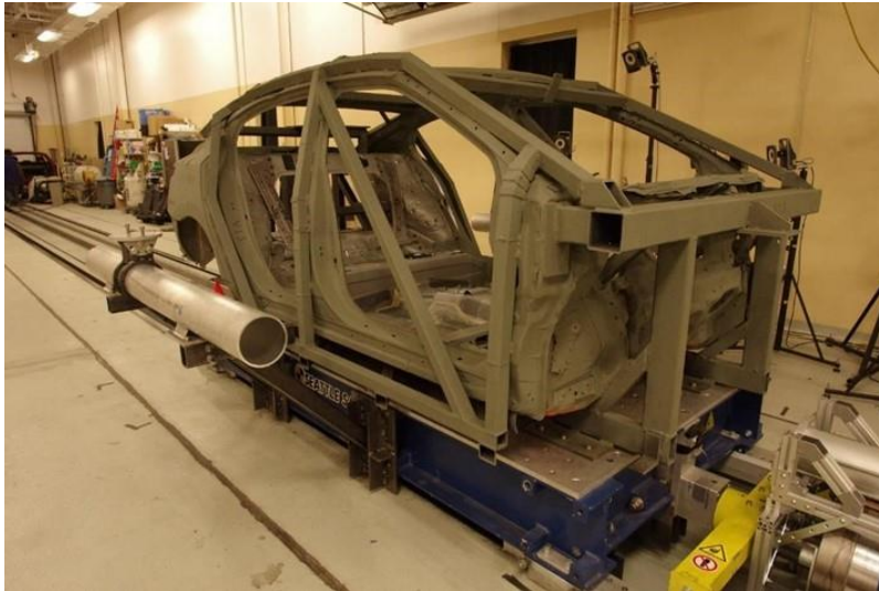
Figure 1. Completed buck (vehicle V15) on the sled.
