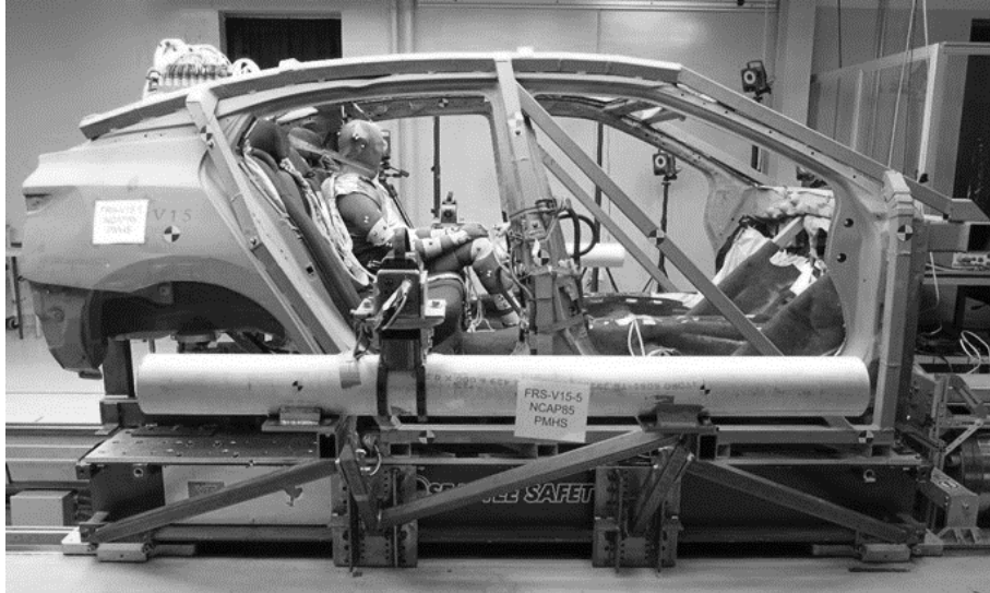
Figure 4. Final setup for a PMHS test in Vehicle V15. The PMHS is seated in the rear left outboard seat of the vehicle buck.
