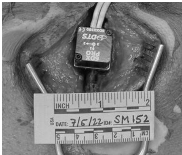
Figure 9. A DTS 6DOF assembly mounted to a spine block before being shrouded.
