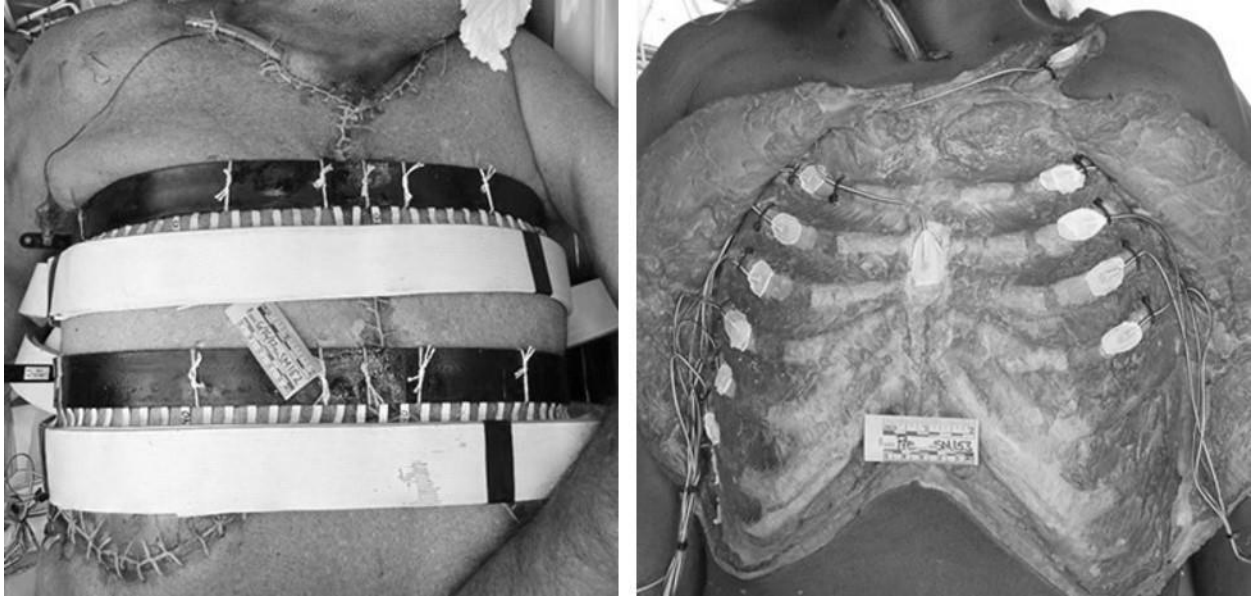
Figure 11. The chest bands positioned at the level of rib 4 and the xiphoid process (left) and the locations of the strain gages on the ribs, sternum, and left clavicle.
