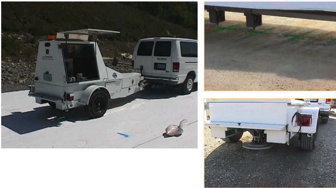
Figure A-11. Falling Weight Deflectometer System
