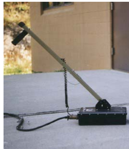
Ground Coupled System (900MHz)
