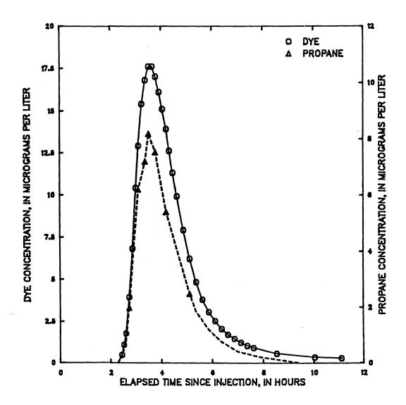
Figure 54 -- Dye and propane concentration from hydrocarbon gas tracer measurements made on Middle Fork Beargrass Creek, downstream end of reach A (upstream end of reach B), May 16, 1985 tracer injection
