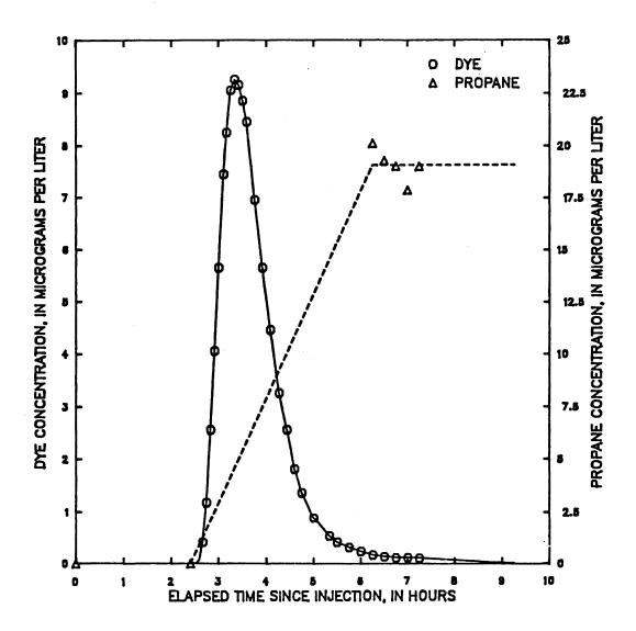
Figure 67 -- Dye and propane concentration from hydrocarbon gas tracer measurements made on Middle Fork Beargrass Creek, downstream end of reach D, April 19, 1985 tracer injection
