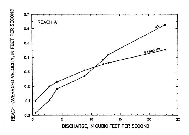
Figure 30 -- Comparison of mean velocity determined by three different methods for reach A of the Middle Fork Beargrass Creek, from tracer measurements made between April 18, 1985 and September 18, 1985
