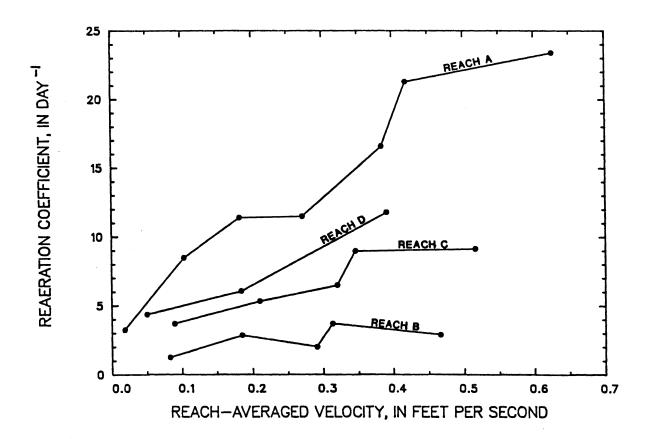
Figure 39 -- Reaeration coefficient shown as a function of reachaveraged velocity for reaches of Middle Fork Beargrass Creek, from tracer measurements made from April 18, 1985 through September 18, 1985
