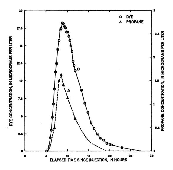
Figure 51 -- Dye and propane concentration from hydrocarbon gas tracer measurements made on Middle Fork Beargrass Creek, downstream end of reach A (upstream end of reach B). May 8, 1985 tracer injection
