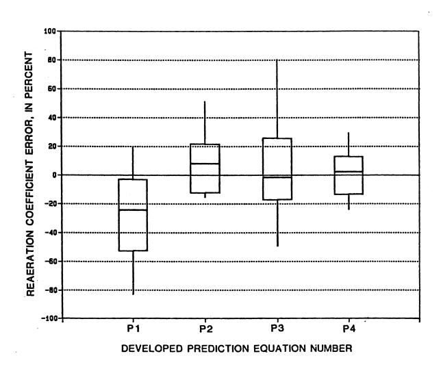
Figure 46 -- Schematic box plots of reaeration coefficient estimates using developed prediction equations and hydrocarbon gas tracer measurement data from reaches of Middle Fork Beargrass Creek
