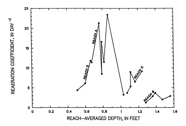
Figure 40 -- Reaeration coefficient shown as a function of reachaveraged depth for reaches of Middle Fork Beargrass Creek, from tracer measurements made from April 18, 1985 through September 18, 1985
