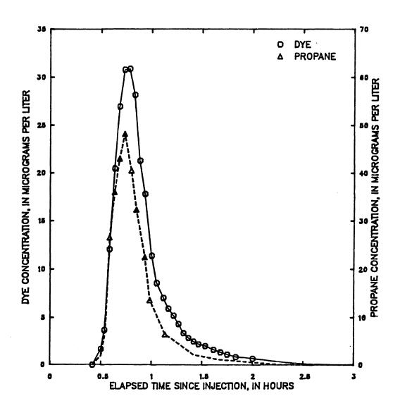
Figure 59 -- Dye and propane concentration from hydrocarbon gas tracer measurements made on Middle Fork Beargrass Creek, upstream end of reach A (upstream end of reach C), June 14, 1985 tracer injection
