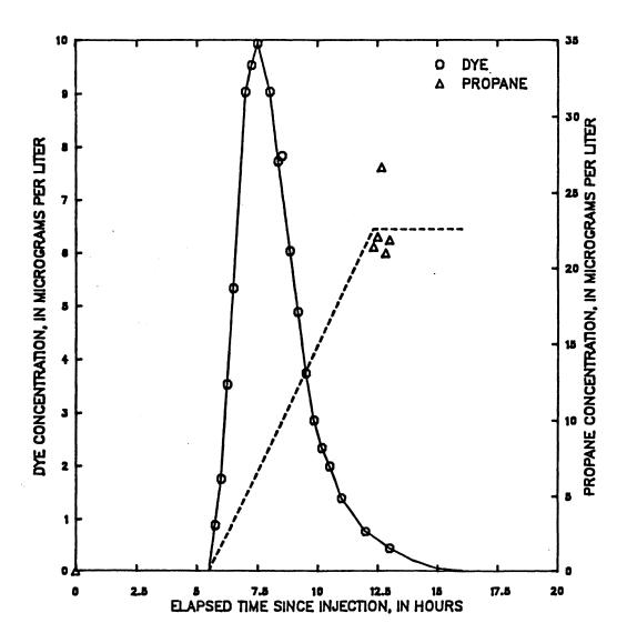
Figure 26 -- Dye and propane concentration from hydrocarbon gas tracer measurements made on Middle Fork Beargrass Creek, downstream end of reach D, May 7, 1985 tracer injection
