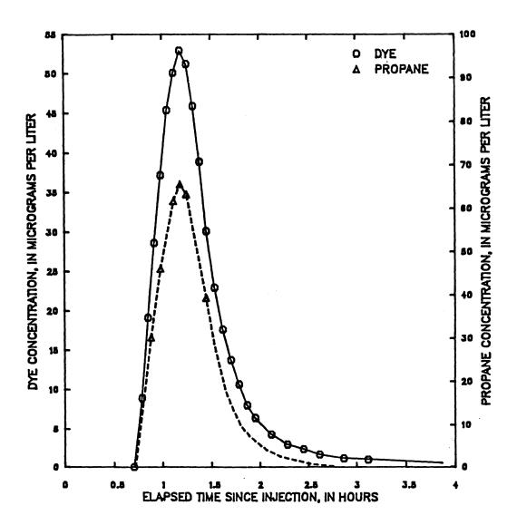
Figure 22 -- Dye and propane concentration from hydrocarbon gas tracer measurements made on Middle Fork Beargrass Creek, upstream end of reach A (upstream end of reach C), May 16, 1985 tracer injection
