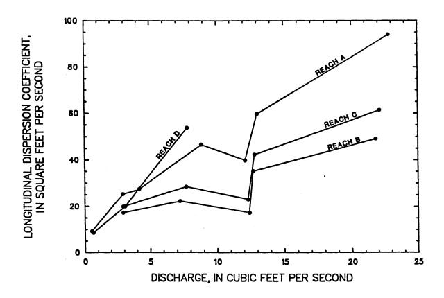
Figure 16 -- Reach-averaged dispersion coefficient shown as a function of discharge for reaches of Middle Fork Beargrass Creek, from tracer measurements made from April 18, 1985 through September 18, 1985
