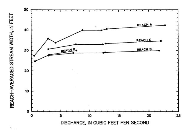
Figure 12 -- Reach-averaged width shown as a function of discharge for reaches of Middle Fork Beargrass Creek, from tracer measurements made from April 18, 1985 through September 18, 1985
