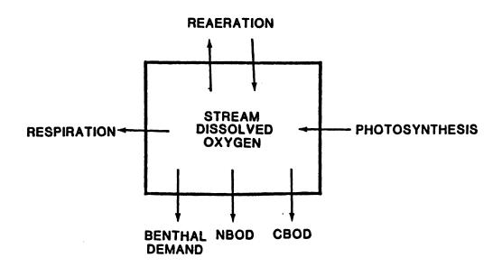
Figure 1 -- Simplified dissolved-oxygen budget for a stream in contact with the atmosphere
