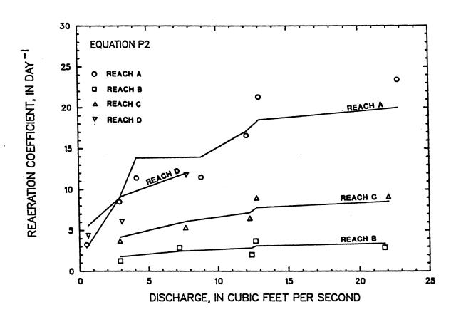
Figure 43 -- Comparison of field-measured reaeration coefficients with those predicted using developed equation, P2
