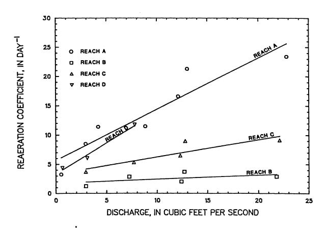
Figure 28 -- Linear relations between the reaeration coefficient and discharge for reaches of Middle Fork Beargrass Creek, from hydrocarbon gas tracer measurements made from April 18, 1985 through September 18, 1985
