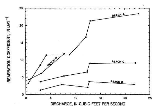
Figure 27 -- Reaeration coefficient shown as a function of discharge for reaches of Middle Fork Beargrass Creek, from tracer measurements made from April 18, 1985 through September 18, 1985
