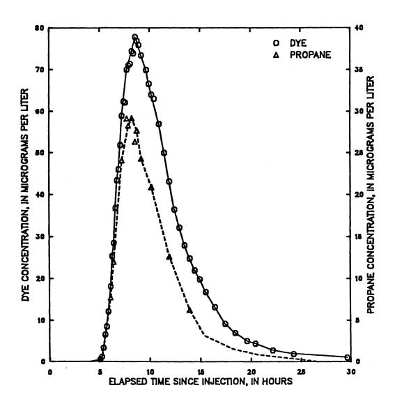
Figure 64 -- Dye and propane concentration from hydrocarbon gas tracer measurements made on Middle Fork Beargrass Creek, upstream end of reach A, September 17, 1985 tracer injection
