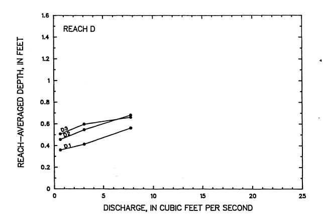
Figure 37 -- Comparison of mean depth determined by three different methods for reach D of the Middle Fork Beargrass Creek, from tracer measurements made between April 18, 1985 and September 18, 1985
