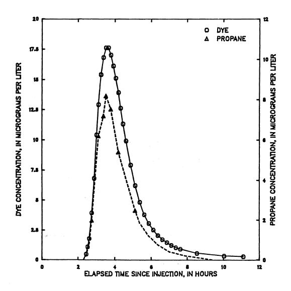
Figure 23 -- Dye and propane concentration from hydrocarbon gas tracer measurements made on Middle Fork Beargrass Creek, downstream end of reach A (upstream end of reach B), May 16, 1985 tracer injection
