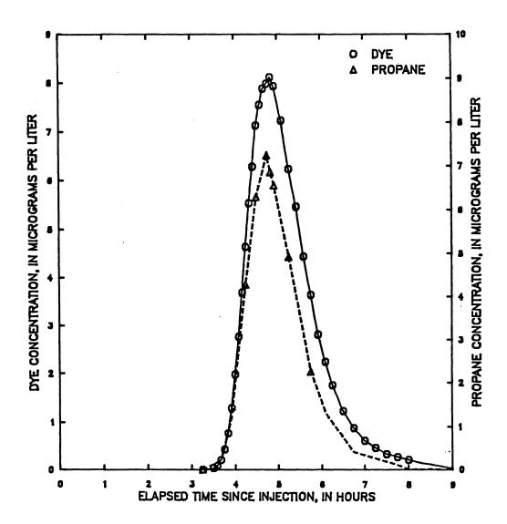
Figure 58 -- Dye and propane concentration from hydrocarbon gas tracer measurements made on Middle Fork Beargrass Creek, downstream end of reach B (downstream end of reach C), May 24, 1985 tracer injection
