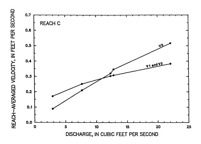
Figure 32 -- Comparison of mean velocity determined by three different methods for reach C of the Middle Fork Beargrass Creek, from tracer measurements made between April 18, 1985 and September 18, 1985
