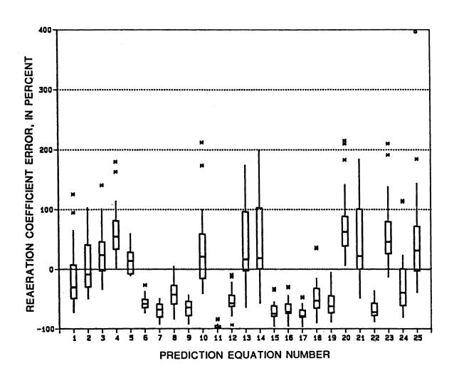
Figure 29 -- Schematic box plots of reaeration coefficient estimates using selected prediction equations and hydrocarbon gas tracer measurement data from reaches of Middle Fork Beargrass Creek
