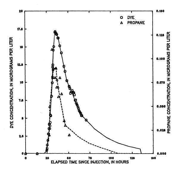
Figure 65 -- Dye and propane concentration from hydrocarbon gas tracer measurements made on Middle Fork Beargrass Creek, downstream end of reach A, September 17, 1985 tracer injection
