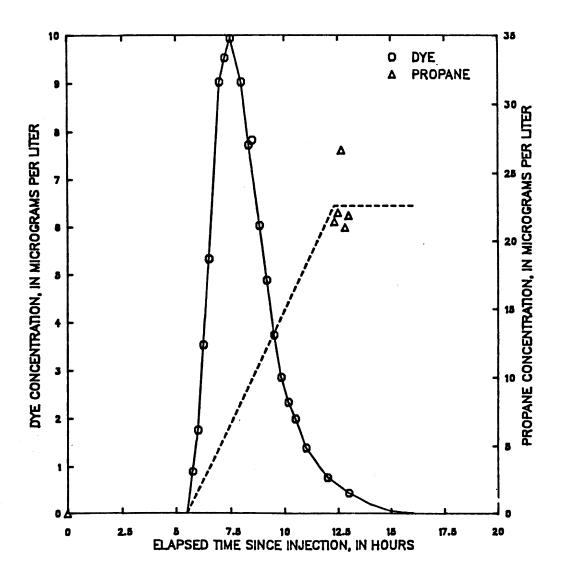
Figure 69 -- Dye and propane concentration from hydrocarbon gas tracer measurements made on Middle Fork Beargrass Creek, downstream end of reach D, May 7, 1985 tracer injection
