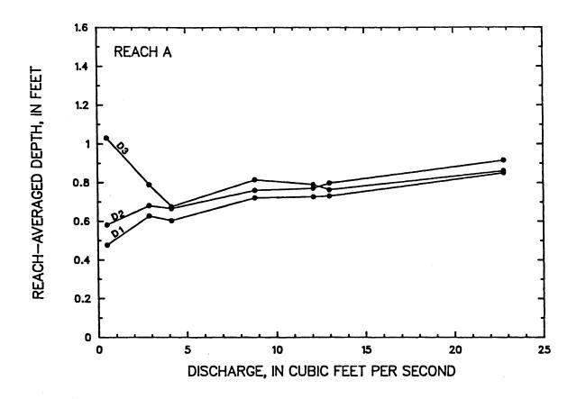
Figure 34 -- Comparison of mean depth determined by three different methods for reach A of the Middle Fork Beargrass Creek, from tracer measurements made between April 18, 1985 and September 18, 1985
