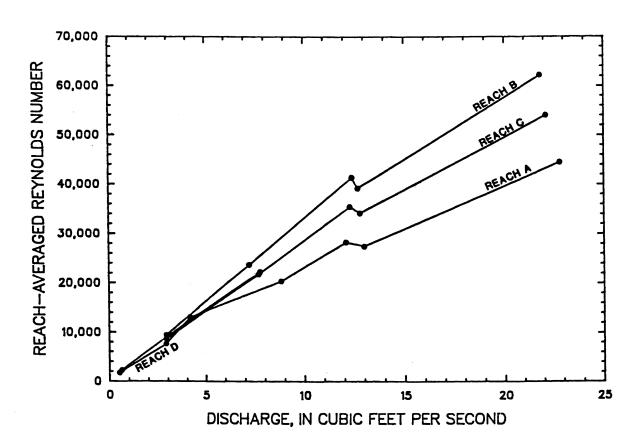
Figure 18 -- Reach-averaged Reynolds number shown as a function of discharge for reaches of Middle Fork Beargrass Creek, from tracer measurements made from April 18, 1985 through September 18, 1985
