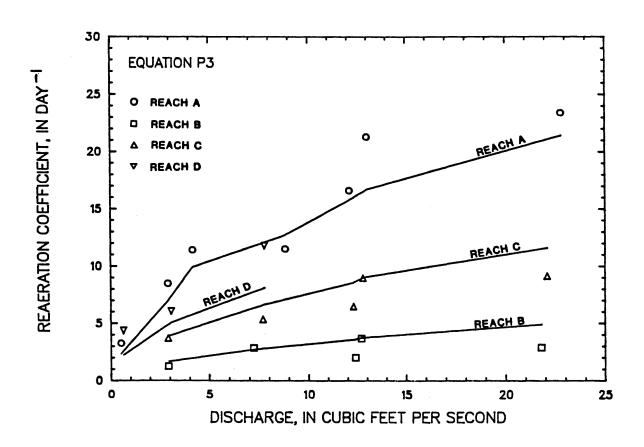
Figure 44 -- Comparison of field-measured reaeration coefficients with those predicted using developed equation, P3
