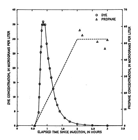
Figure 66 -- Dye and propane concentration from hydrocarbon gas tracer measurements made on Middle Fork Beargrass Creek, upstream end of reach D, April 19, 1985 tracer injection
