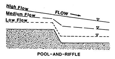
Figure 3 -- Stylized profiles for pool-and-riffle and channel-controlled stream reaches under various flow conditions
