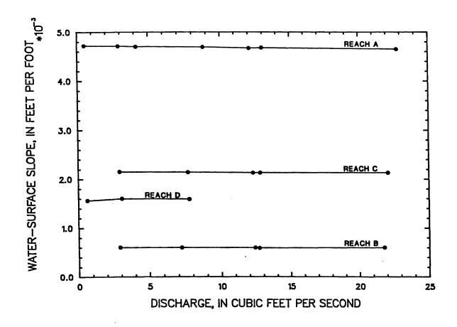
Figure 9 -- Reach-averaged water-surface slope shown as a function of discharge for reaches of Middle Fork Beargrass Creek, from tracer measurements made from April 18, 1985 through September 18, 1985
