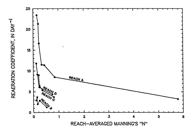
Figure 78 -- Reaeration coefficient shown as a function of reachaveraged Mannings "n" values for reaches of Middle Fork Beargrass Creek, from tracer measurements made from April 18, 1985 through September 18, 1985
