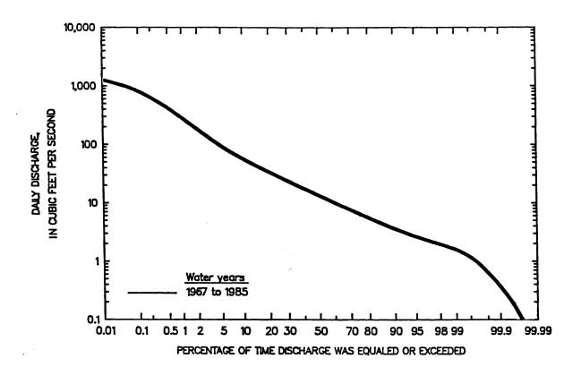
Figure 5 -- Flow duration curve for daily mean discharges for Middle Fork Beargrass Creek, 1966-1985
