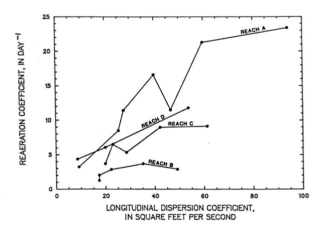
Figure 41 -- Reaeration coefficient shown as a function of reachaveraged dispersion coefficient for reaches of Middle Fork Beargrass Creek, from tracer measurements made from April 18, 1985 through September 18, 1985
