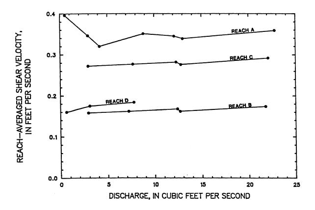
Figure 15 -- Reach-averaged shear velocity shown as a function of discharge for reaches of Middle Fork Beargrass Creek, from tracer measurements made from April 18, 1985 through September 18, 1985
