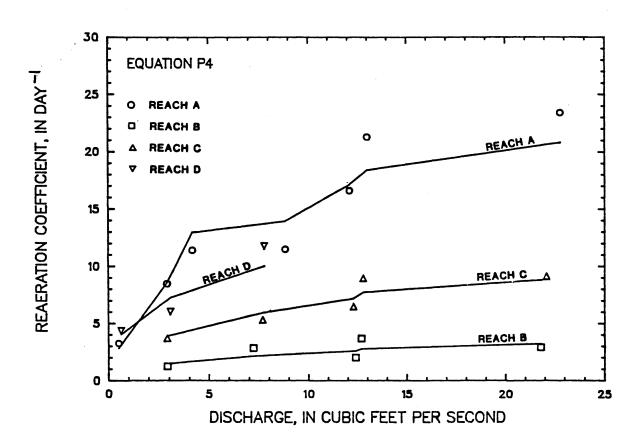
Figure 45 -- Comparison of field-measured reaeration coefficients with those predicted using developed equation, P4
