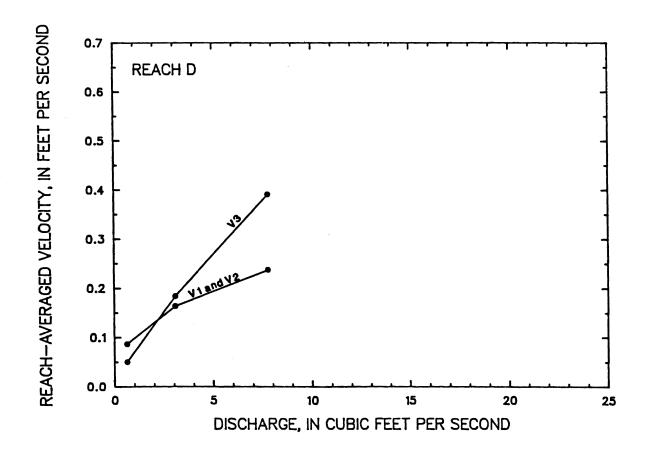
Figure 33 -- Comparison of mean velocity determined by three different methods for reach D of the Middle Fork Beargrass Creek, from tracer measurements made between April 18, 1985 and September 18, 1985
