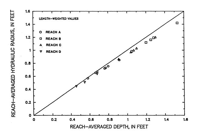
Figure 8 -- Comparison of reach-averaged depth and reach-averaged hydraulic radius determined from length-weighted hydraulic measurements
