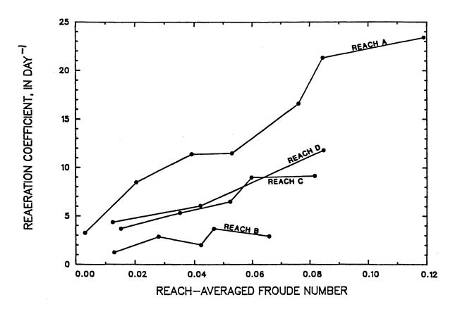
Figure 74 -- Reaeration coefficient shown as a function of reachaveraged Froude number for reaches of Middle Fork Beargrass Creek, from tracer measurements made from April 18, 1985 through September 18, 1985
