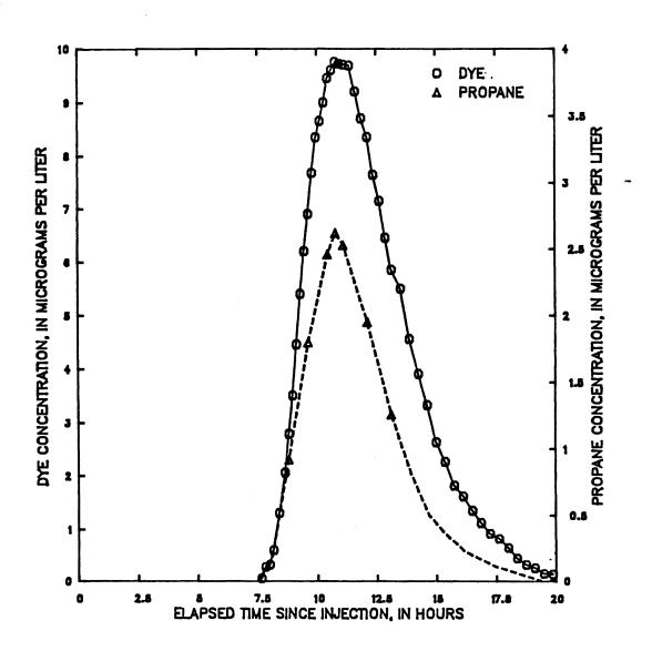
Figure 55 -- Dye and propane concentration from hydrocarbon gas tracer measurements made on Middle Fork Beargrass Creek, downstream end of reach B (downstream end of reach C), May 16, 1985 tracer injection
