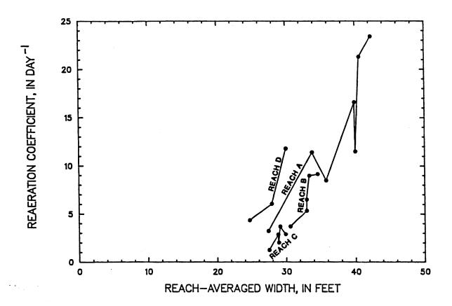
Figure 72 -- Reaeration coefficient shown as a function of reachaveraged width for reaches of Middle Fork Beargrass Creek, from tracer measurements made from April 18, 1985 through September 18, 1985
