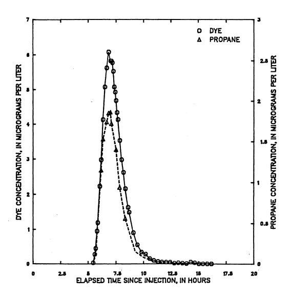
Figure 61 -- Dye and propane concentration from hydrocarbon gas tracer measurements made on Middle Fork Beargrass Creek, downstream end of reach B (downstream end of reach C), June 14, 1985 tracer injection
