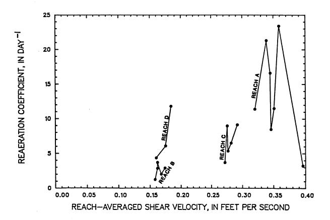
Figure 75 -- Reaeration coefficient shown as a function of reachaveraged shear velocity for reaches of Middle Fork Beargrass Creek, from tracer measurements made from April 18, 1985 through September 18, 1985
