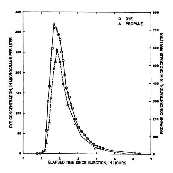
Figure 70 -- Dye and propane concentration from hydrocarbon gas tracer measurements made on Middle Fork Beargrass Creek, upstream end of reach D, September 18, 1985 tracer injection
