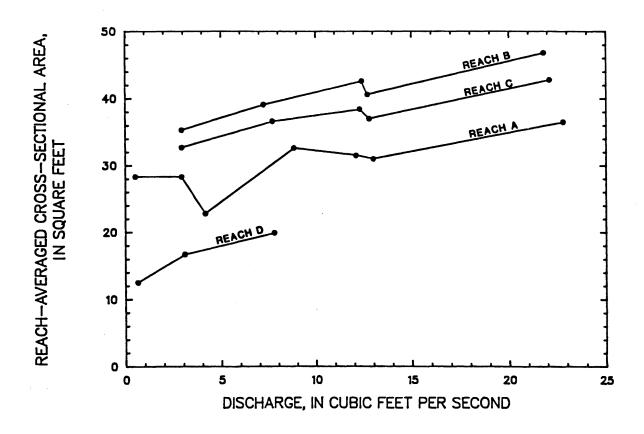
Figure 13 -- Reach-averaged cross-sectional area shown as a function of discharge for reaches of Middle Fork Beargrass Creek, from tracer measurements made from April 18, 1985 through September 18, 1985
