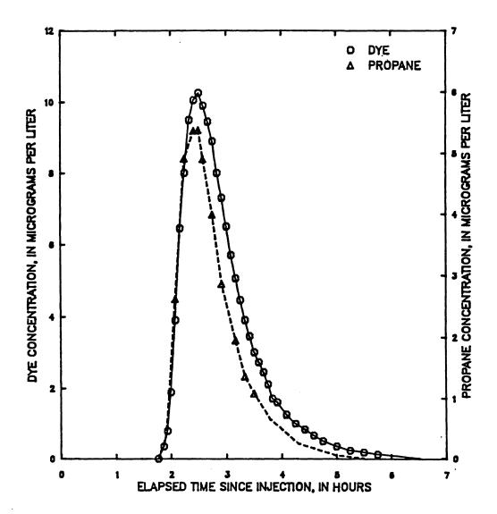
Figure 60 -- Dye and propane concentration from hydrocarbon gas tracer measurements made on Middle Fork Beargrass Creek, downstream end of reach A (upstream end of reach B), June 14, 1985 tracer injection
