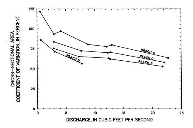
Figure 20 -- Coefficient of variation of cross-sectional area as a function of discharge for reaches of Middle Fork Beargrass Creek, from tracer measurements made from April 18, 1985 through September 18, 1985
