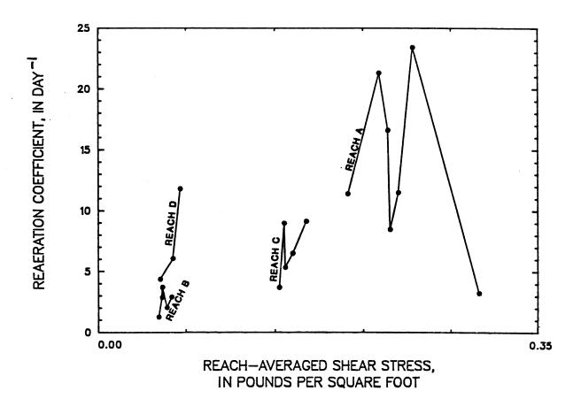
Figure 76 -- Reaeration coefficient shown as a function of reachaveraged shear stress for reaches of Middle Fork Beargrass Creek, from tracer measurements made from April 18, 1985 through September 18, 1985
