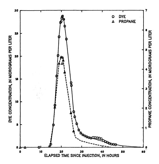
Figure 71 -- Dye and propane concentration from hydrocarbon gas tracer measurements made on Middle Fork Beargrass Creek, downstream end of reach D, September 18, 1985 tracer injection
