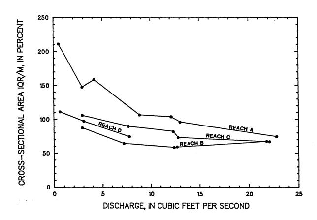
Figure 21 -- Interquartile range divided by the median (expressed as a percent) value of cross-sectional area as a function of discharge for reaches of Middle Fork Beargrass Creek, from tracer measurements made from April 18, 1985 through September 18, 1985
