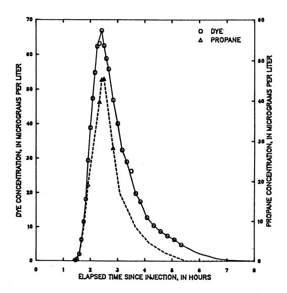
Figure 50 -- Dye and propane concentration from hydrocarbon gas tracer measurements made on Middle Fork Beargrass Creek, upstream end of reach A (upstream end of reach C), May 8, 1985 tracer injection
