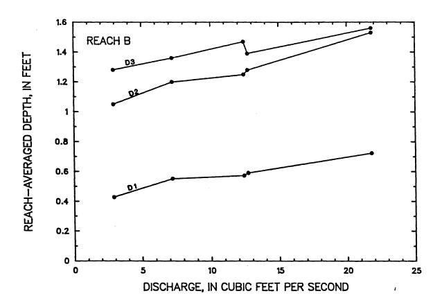
Figure 35 -- Comparison of mean depth determined by three different methods for reach B of the Middle Fork Beargrass Creek, from tracer measurements made between April 18, 1985 and September 18, 1985
