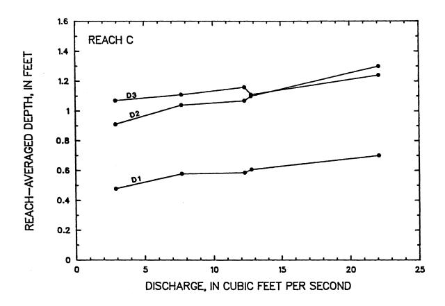
Figure 36 -- Comparison of mean depth determined by three different methods for reach C of the Middle Fork Beargrass Creek, from tracer measurements made between April 18, 1985 and September 18, 1985
