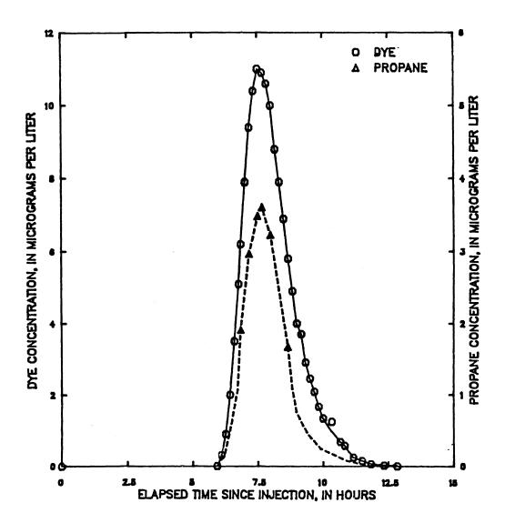
Figure 49 -- Dye and propane concentration from hydrocarbon gas tracer measurements made on Middle Fork Beargrass Creek, downstream end of reach B (downstream end of reach C), April 18, 1985 tracer injection
