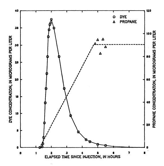
Figure 25 -- Dye and propane concentration from hydrocarbon gas tracer measurements made on Middle Fork Beargrass Creek, upstream end of reach D, May 7, 1985 tracer injection
