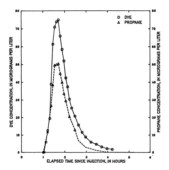
Figure 62 -- Dye and propane concentration from hydrocarbon gas tracer measurements made on Middle Fork Beargrass Creek, upstream end of reach A, August 19, 1985 tracer injection
