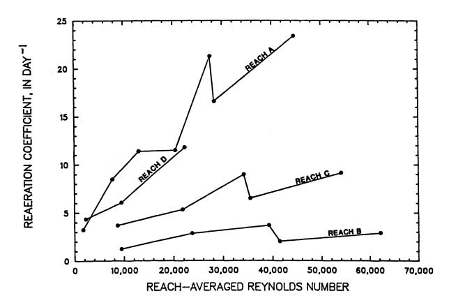
Figure 77 -- Reaeration coefficient shown as a function of reachaveraged Reynolds number for reaches of Middle Fork Beargrass Creek, from tracer measurements made from April 18, 1985 through September 18, 1985
