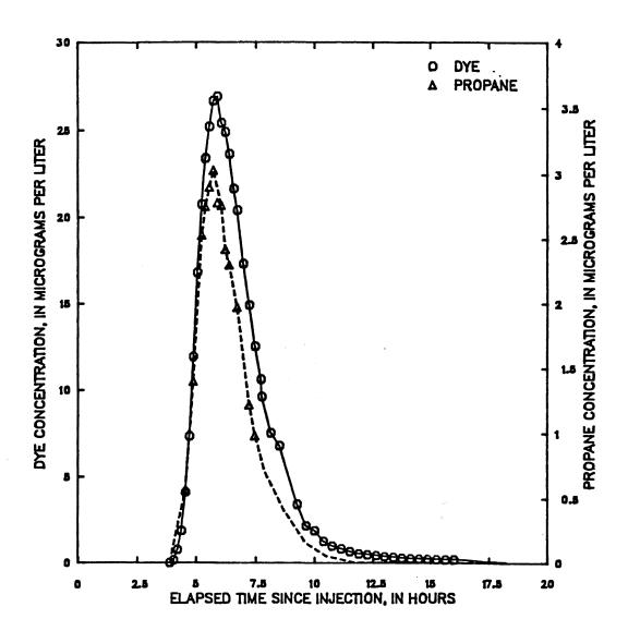
Figure 63 -- Dye and propane concentration from hydrocarbon gas tracer measurements made on Middle Fork Beargrass Creek, downstream end of reach A, August 19, 1985 tracer injection
