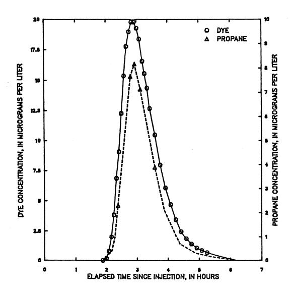
Figure 48 -- Dye and propane concentration from hydrocarbon gas tracer measurements made on Middle Fork Beargrass Creek, downstream end of reach A (upstream end of reach B), April 18, 1985 tracer injection
