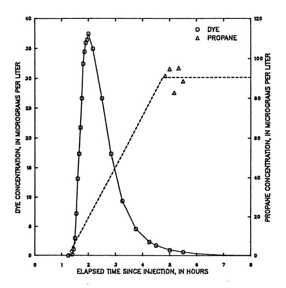
Figure 68 -- Dye and propane concentration from hydrocarbon gas tracer measurements made on Middle Fork Beargrass Creek, upstream end of reach D, May 7, 1985 tracer injection
