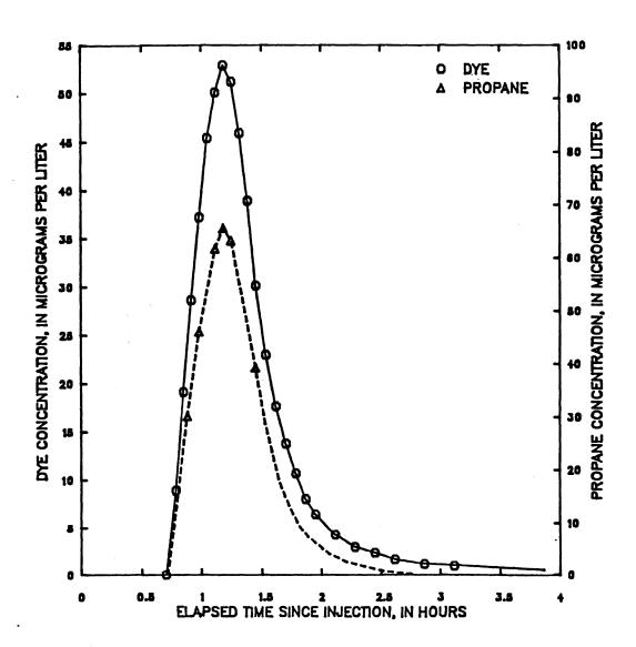
Figure 53 -- Dye and propane concentration from hydrocarbon gas tracer measurements made on Middle Fork Beargrass Creek, upstream end of reach A (upstream end of reach C), May 16, 1985 tracer injection
