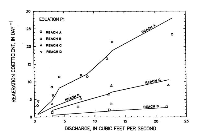
Figure 42 -- Comparison of field-measured reaeration coefficients with those predicted using developed equation, P1
