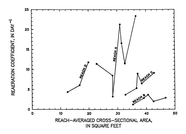
Figure 73 -- Reaeration coefficient shown as a function of reachaveraged cross-sectional area for reaches of Middle Fork Beargrass Creek, from tracer measurements made from April 18, 1985 through September 18, 1985
