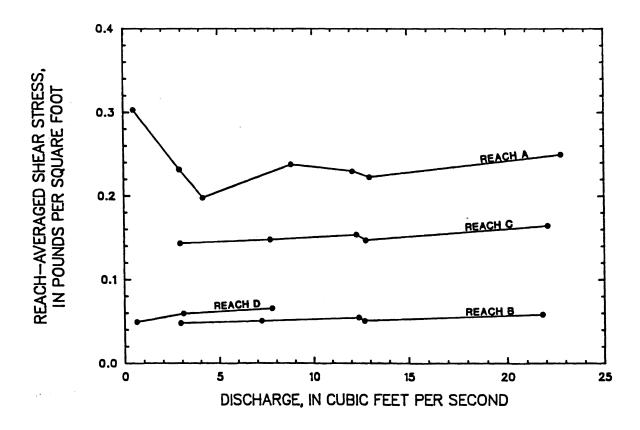
Figure 17 -- Reach-averaged shear stress shown as a function of discharge for reaches of Middle Fork Beargrass Creek, from tracer measurements made from April 18, 1985 through September 18, 1985
