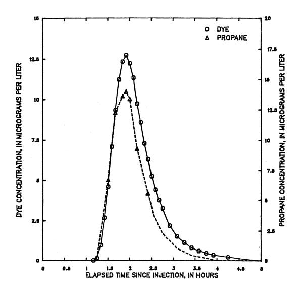
Figure 57 -- Dye and propane concentration from hydrocarbon gas tracer measurements made on Middle Fork Beargrass Creek, downstream end of reach A (upstream end of reach B), May 24, 1985 tracer injection
