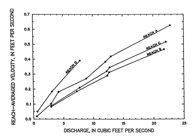
Figure 10 -- Reach-averaged velocity shown as a function of discharge for reaches of Middle Fork Beargrass Creek, from tracer measurements made from April 18, 1985 through September 18, 1985
