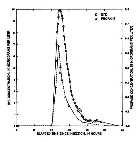
Figure 52 -- Dye and propane concentration from hydrocarbon gas tracer measurements made on Middle Fork Beargrass Creek, downstream end of reach B (downstream end of reach C), May 8, 1985 tracer injection
