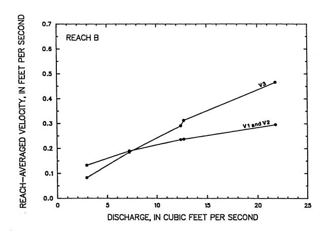
Figure 31 -- Comparison of mean velocity determined by three different methods for reach B of the Middle Fork Beargrass Creek, from tracer measurements made between April 18, 1985 and September 18, 1985
