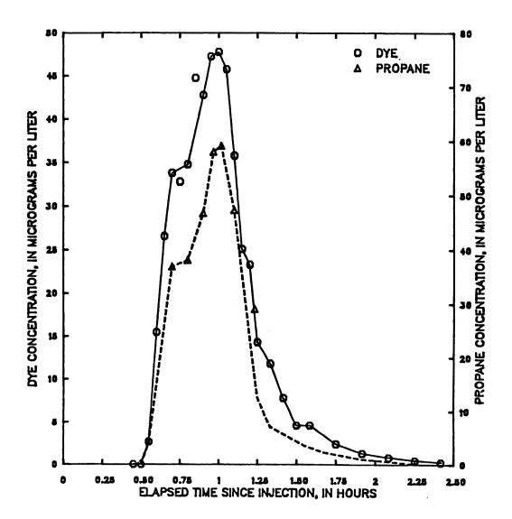
Figure 47 -- Dye and propane concentration from hydrocarbon gas tracer measurements made on Middle Fork Beargrass Creek, upstream end of reach A (upstream end of reach C), April 18, 1985 tracer injection
