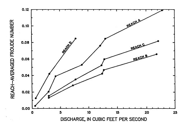
Figure 14 -- Reach-averaged Froude number shown as a function of discharge for reaches of Middle Fork Beargrass Creek, from tracer measurements made from April 18, 1985 through September 18, 1985
