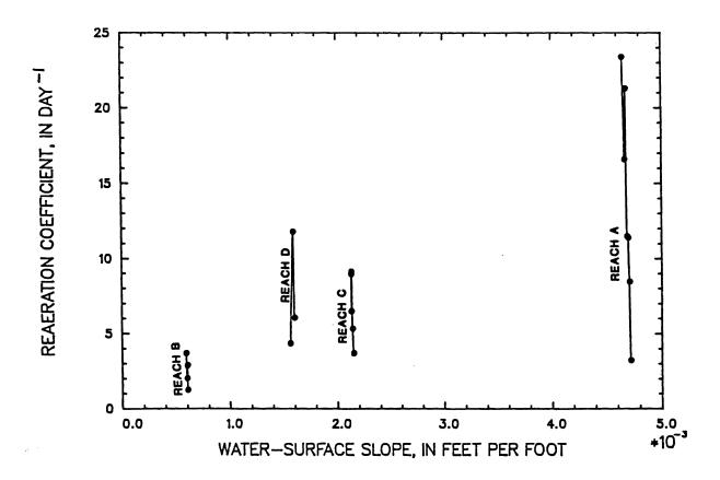
Figure 38 -- Reaeration coefficient shown as a function of reachaveraged water-surface slope for reaches of Middle Fork Beargrass Creek, from tracer measurements made from April 18, 1985 through September 18, 1985
