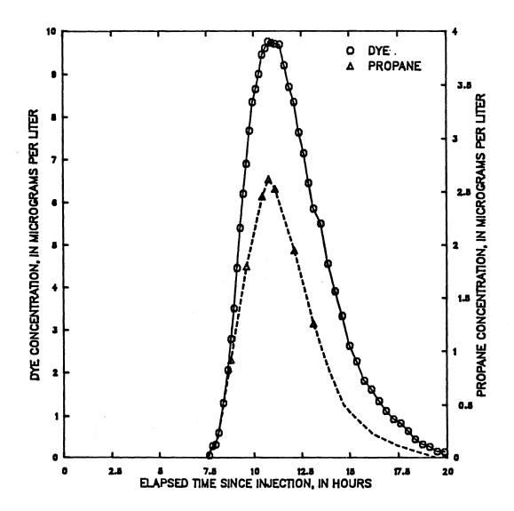
Figure 24 -- Dye and propane concentration from hydrocarbon gas tracer measurements made on Middle Fork Beargrass Creek, downstream end of reach B (downstream end of reach C), May 16, 1985 tracer injection
