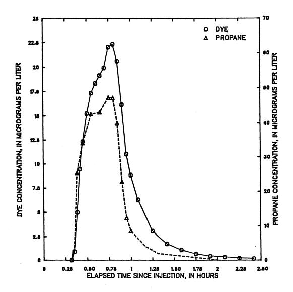
Figure 56 -- Dye and propane concentration from hydrocarbon gas tracer measurements made on Middle Fork Beargrass Creek, upstream end of reach A (upstream end of reach C), May 24, 1985 tracer injection
