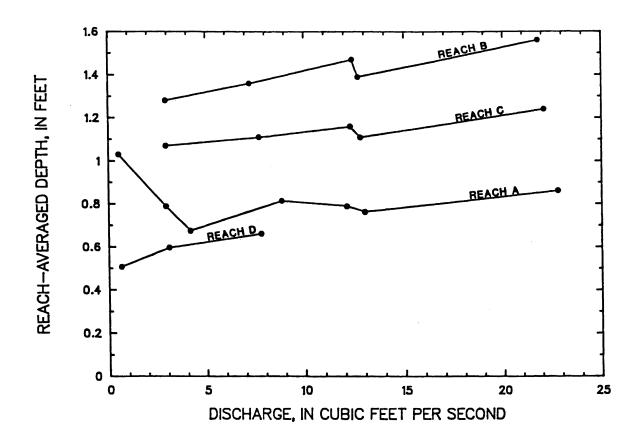
Figure 11 -- Reach-averaged depth shown as a function of discharge for reaches of Middle Fork Beargrass Creek, from tracer measurements made from April 18, 1985 through September 18, 1985
