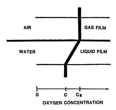
Figure 2 -- Schematic of the surface film theory of gas transfer
