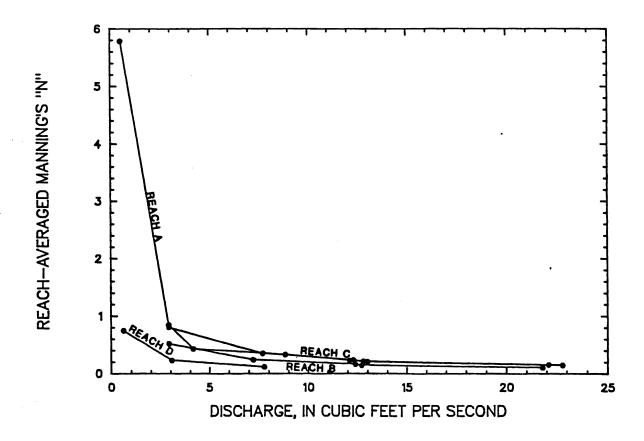
Figure 19 -- Reach-averaged Manning "n" value shown as a function of discharge for reaches of Middle Fork Beargrass Creek, from tracer measurements made from April 18, 1985 through September 18, 1985
