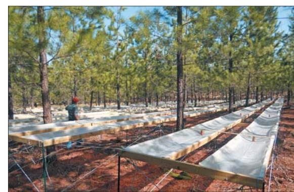
PINEMAP research was conducted at several locations. At a site in Appomattox County, Virginia, plastic troughs reduced rainwater reaching the soil by 33 percent, allowing scientists to simulate how a future climate with less rainfall would affect loblolly pine.
