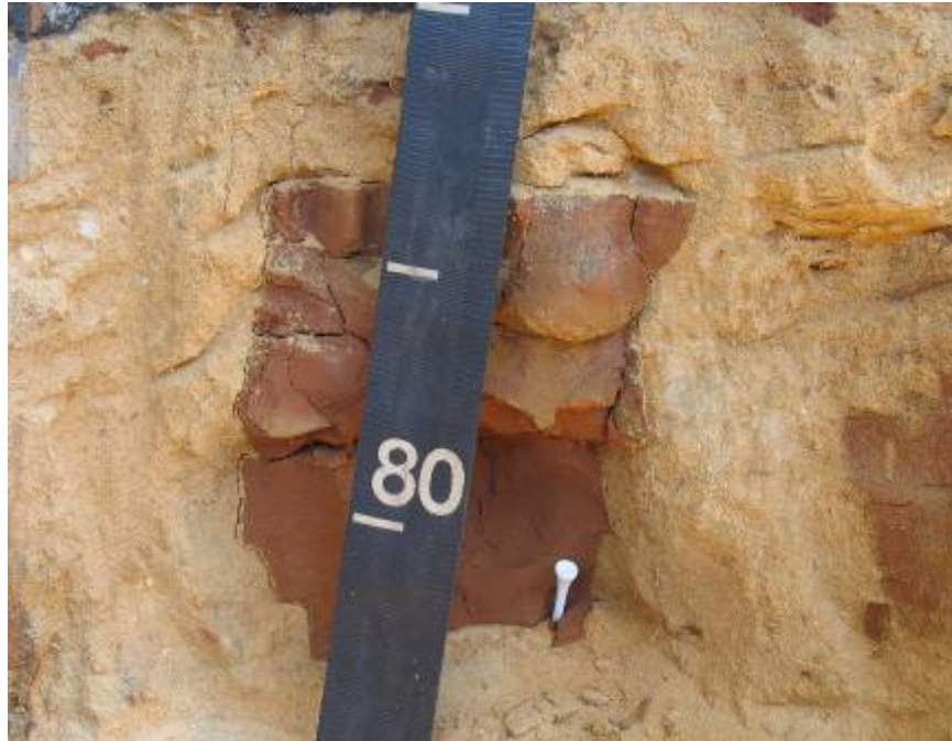
Figure 31. A closer view of Profile 103-2 (Control) showing rounded faces on dewatered chunks of slimes. This overall morphology is most likely the result of dessication of a high slimes layer in the drying surface of a mine pit that was then covered with a fresh layer of sandy tailings.
