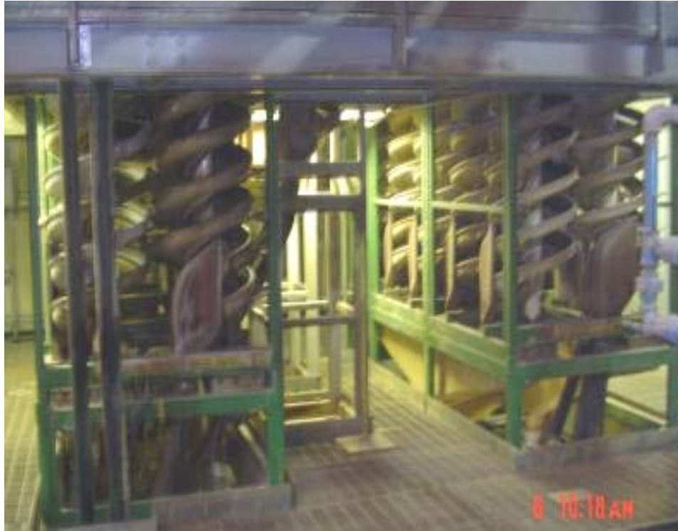
Figure 6. Bank of spirals in wet mill. As the ore passes down the spirals in water, the lighter quartz and non-heavy minerals move to the outside of the spirals while the heavy minerals remain to the inside. The non-heavy mineral fraction (primarily quartz) is sent to the tailings sump to be pumped back to mine pits mixed with slimes. Photo courtesy of Chuck Stilson/Iluka.
