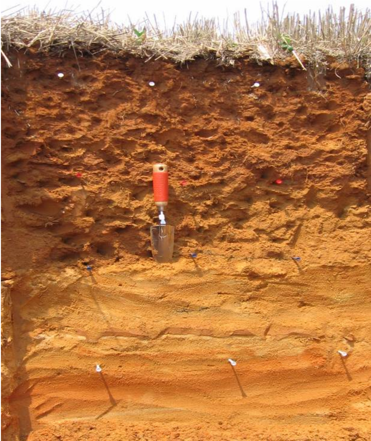
Figure 26. Profile 302-3 (Bio-CT) is a Typic Dystrudept as indicated by weak development of a (Bw) pedogenically-altered horizon (Table 20). This soil classified as an Inceptisol due to the presence of a cambic horizon with > 50% moderate subangular blocky structure between 12 and 44cm. This profile also showed typical sequence of finer textured high slimes material over sandy tailings at depth. Described horizons were ^Ap-^Bw1-^Bw2-^C1-^C2.
