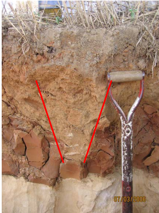
Figure 33. Southern wall of CWRF 101-4 (Ripping traces highlighted in red). Please note the v-shaped ripper trace (out-lined in red) in the upper half of the pit face. Ripping traces were only noted within CWRF 102-3 and 104-5.
