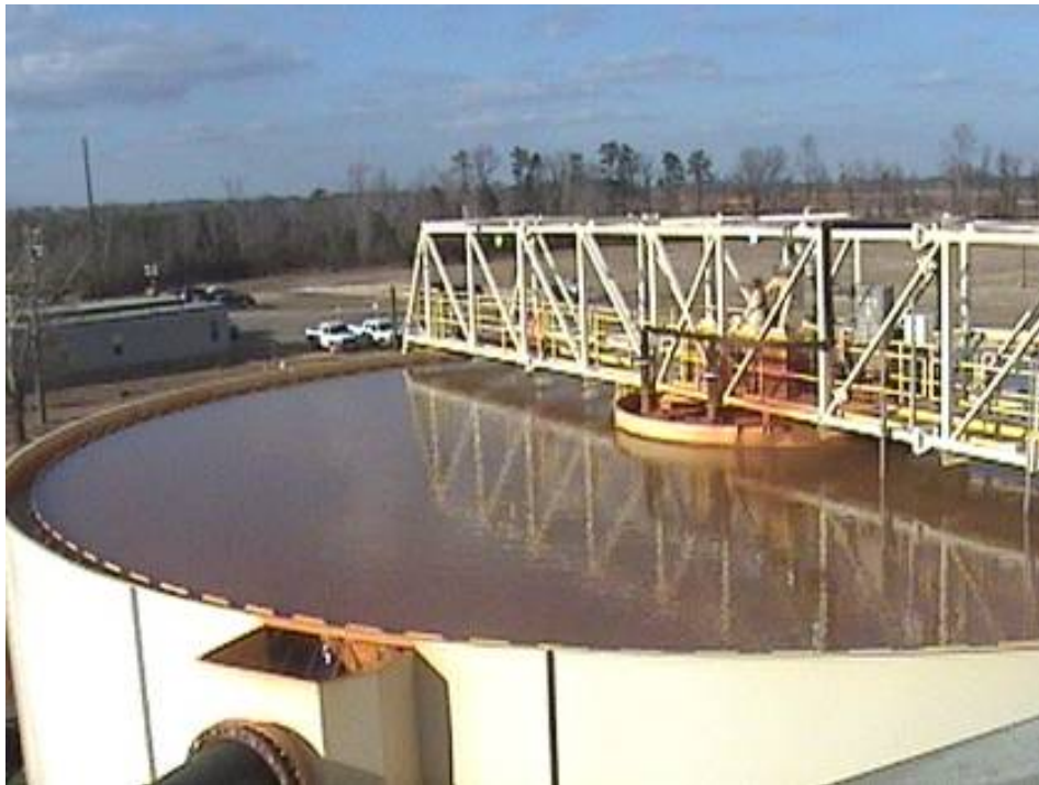
Figure 7. Thickener tank where slimes are flocculated with anionic polymers and fall to bottom where they are removed and combined with tailings to be pumped to backfill mined out pits. Clear water is decanted from the top of the thickener and returned to the wet mill. Photo courtesy of Chuck Stilson/Iluka.
