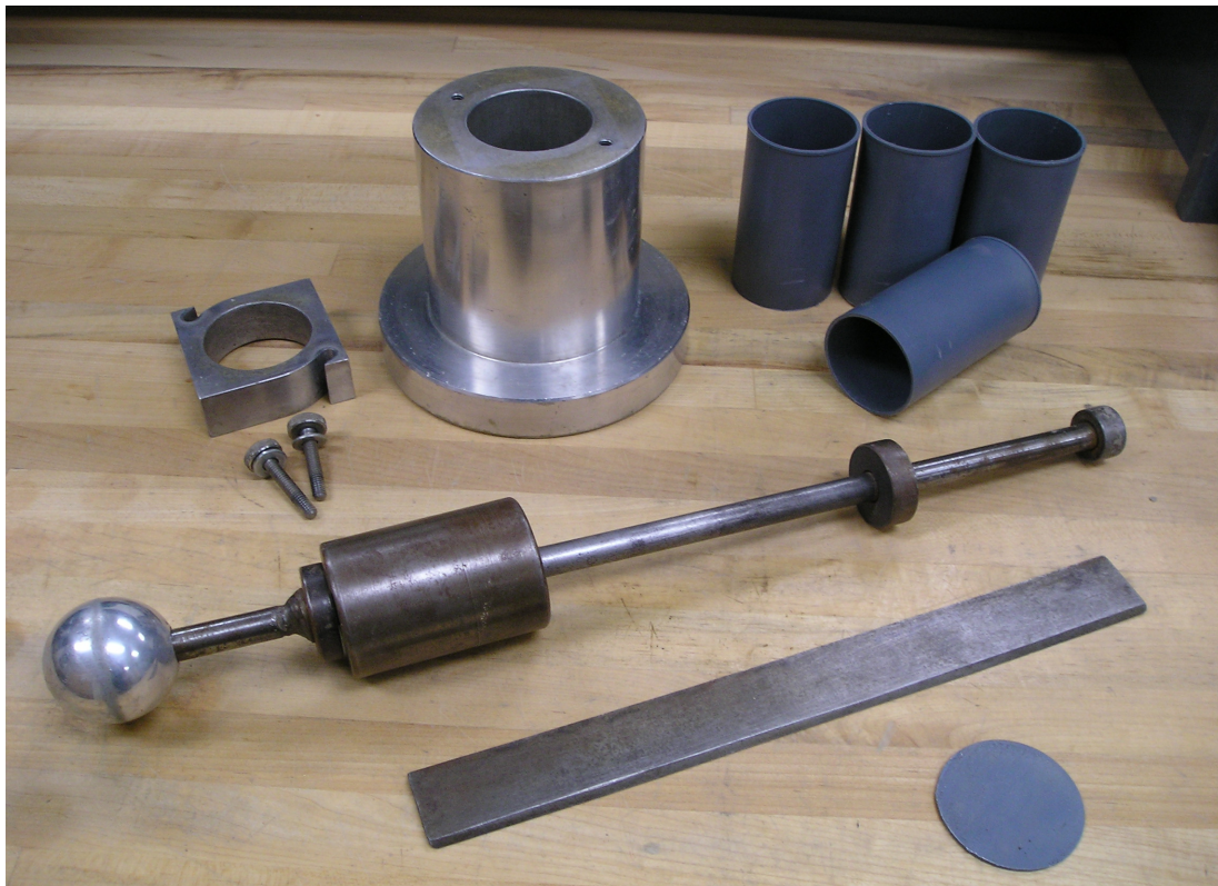
Figure A-3. The “Geiman Cylinder Mold Stand,” retaining ring and screws, the “Geiman Special Hammer,” modified plastic molds, detached plastic bottom, and metal screed.
