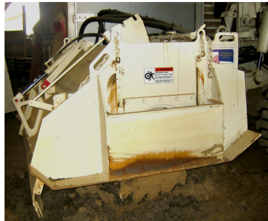
Figure 2-2. Closer view of a pulverizer and its blades. (Photo by James K. Mitchell)
