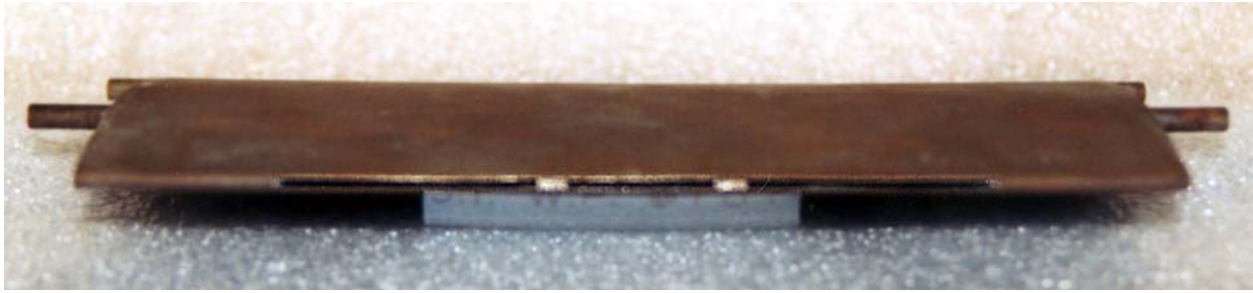
Figure 2-4 Photograph of blade used for testing with trailing edge slot – note the three part division
