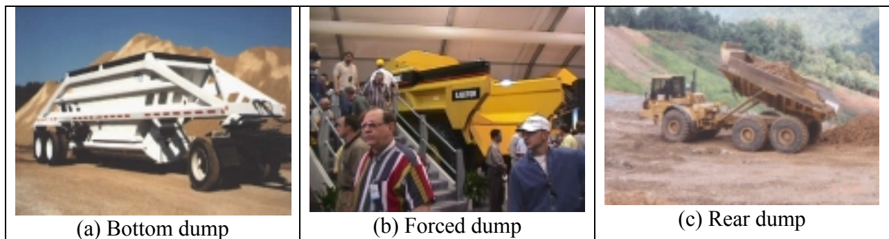
Figure 8-1: Different types of dump mechanisms in a truck
