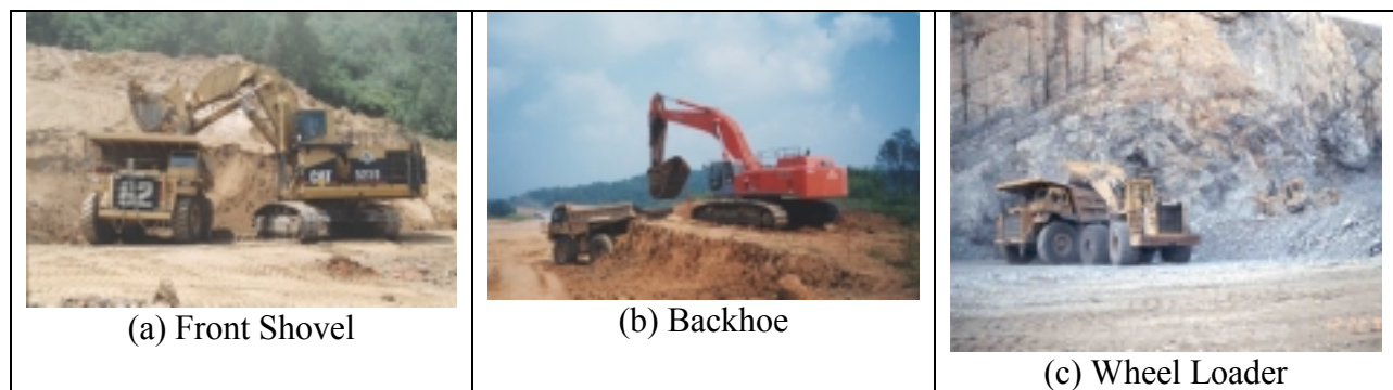
Figure 9-3: Different types of loading methods
