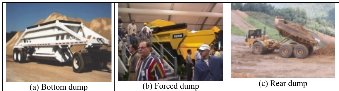
Figure 11-2: Different types of dump mechanisms in a truck
