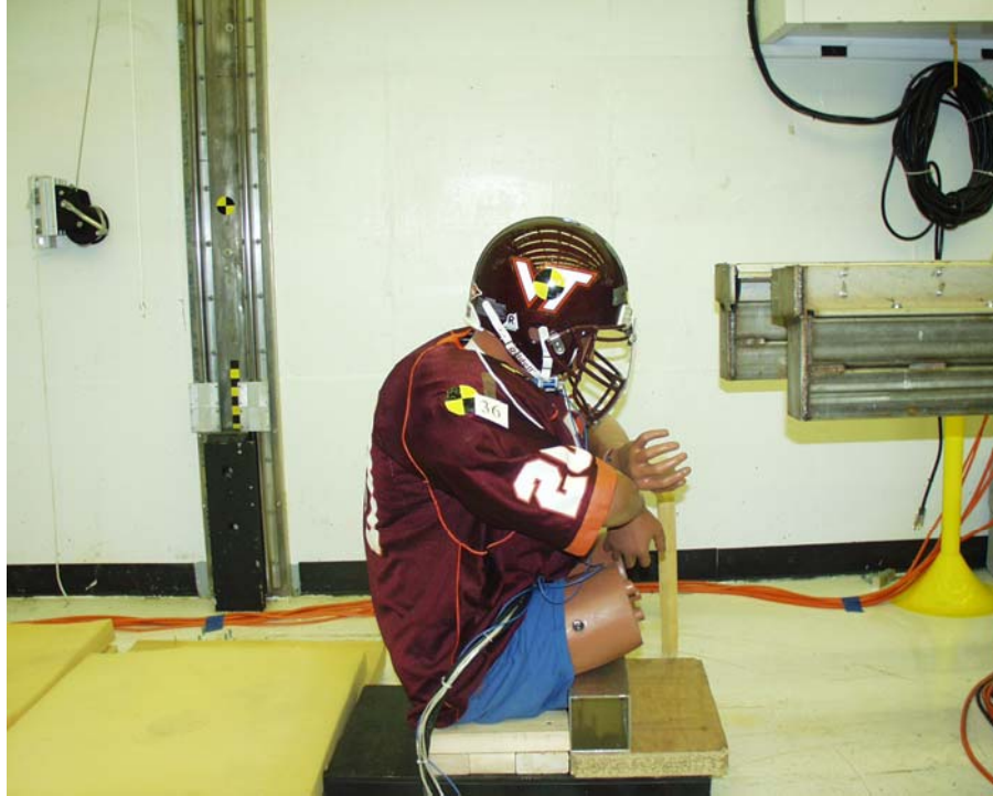
Figure B 3: Side impact location (front view)
