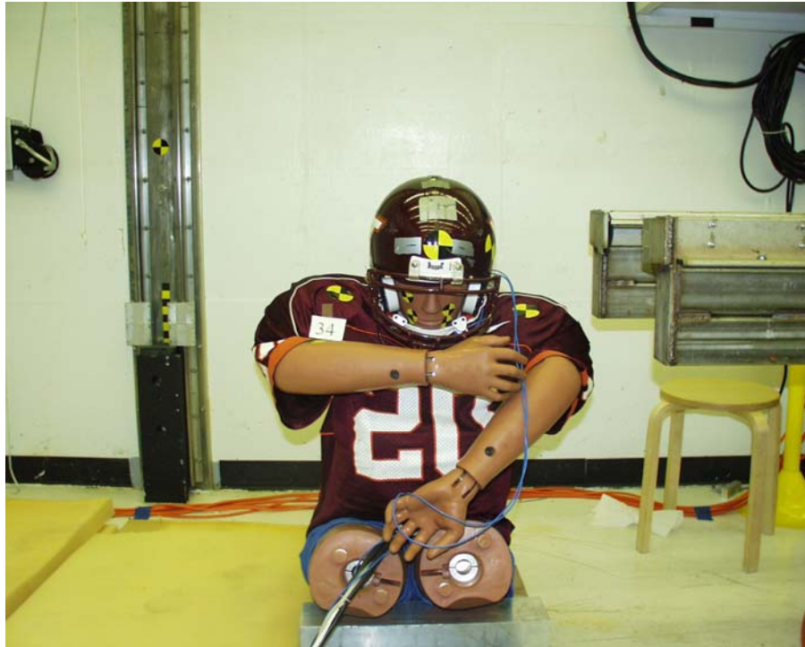
Figure B 1: Side impact location (front view)
