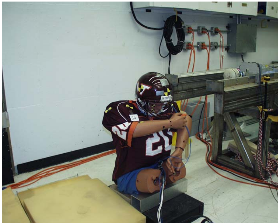
Figure B 2: Side impact location (oblique view)
