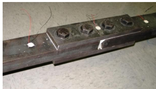
Figure 3.6. PZT patches attached to the switch rod surface
