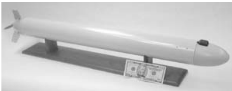
Figure 2.2: Prototype miniature autonomous underwater vehicle
