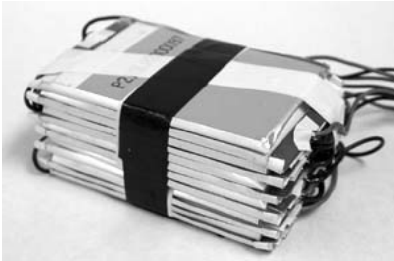
Figure 2.5: Constructed battery stack
