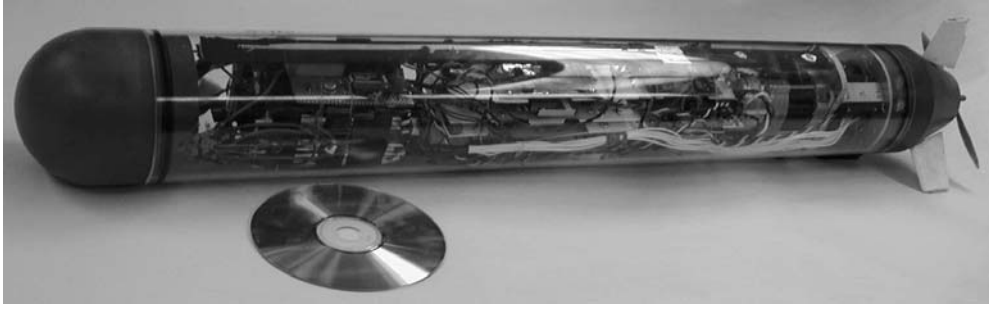
Figure 2.3: VT miniature AUV with clear shell
