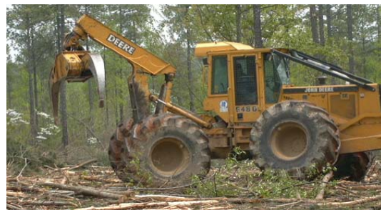
Figure 5. A general mechanized harvesting system consists of a wheeled feller-buncher (photo to left) to fell and bunch trees and then a grapple skidder (photo to right) transports the timber to the landing deck. Photos taken from the College of Natural Resources at Virginia Tech website, www.cnr.vt.edu .
