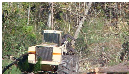
Figure 5. A general mechanized harvesting system consists of a wheeled feller-buncher (photo to left) to fell and bunch trees and then a grapple skidder (photo to right) transports the timber to the landing deck. Photos taken from the College of Natural Resources at Virginia Tech website, www.cnr.vt.edu .
