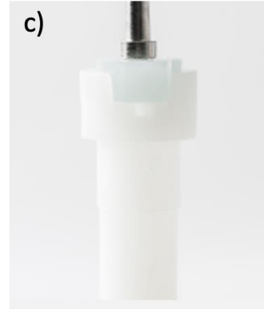
c) 10-mm nylon/ Dorr Oliver cyclone (1.7 L/min) with built-in fitting
