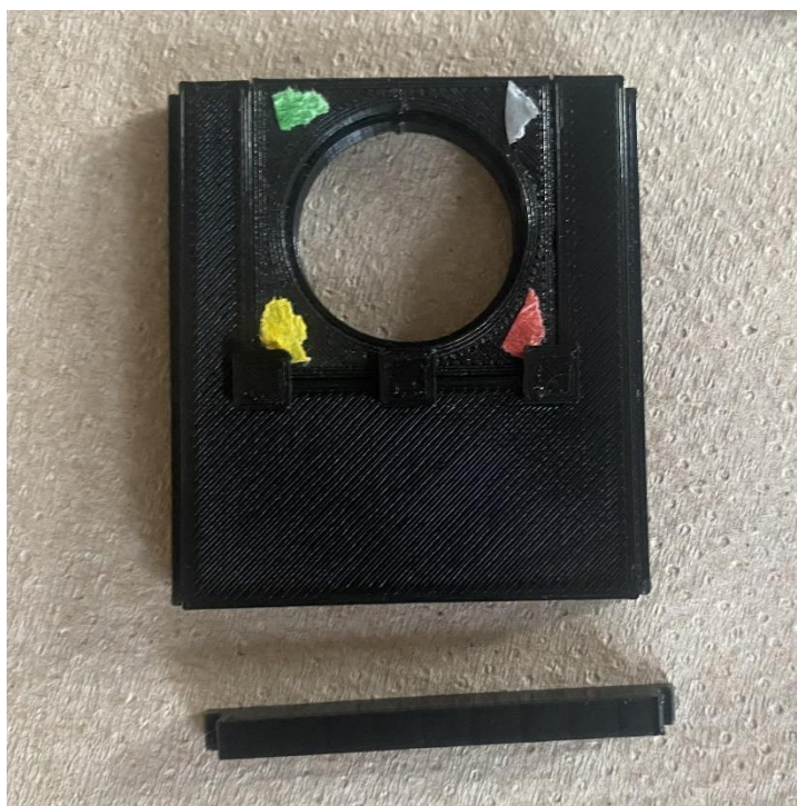
Figure 3.2: 3-D printed 25mm filter holder (above) and 4mm offset spacer.
