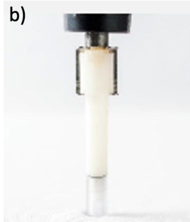
b) CMDPSU (2 L/min), conductive 4-piece cassette
