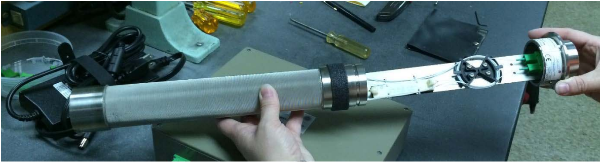
Figure 4.6: Fiber Optic Methane sensor with screen slid off of the FO frame.
