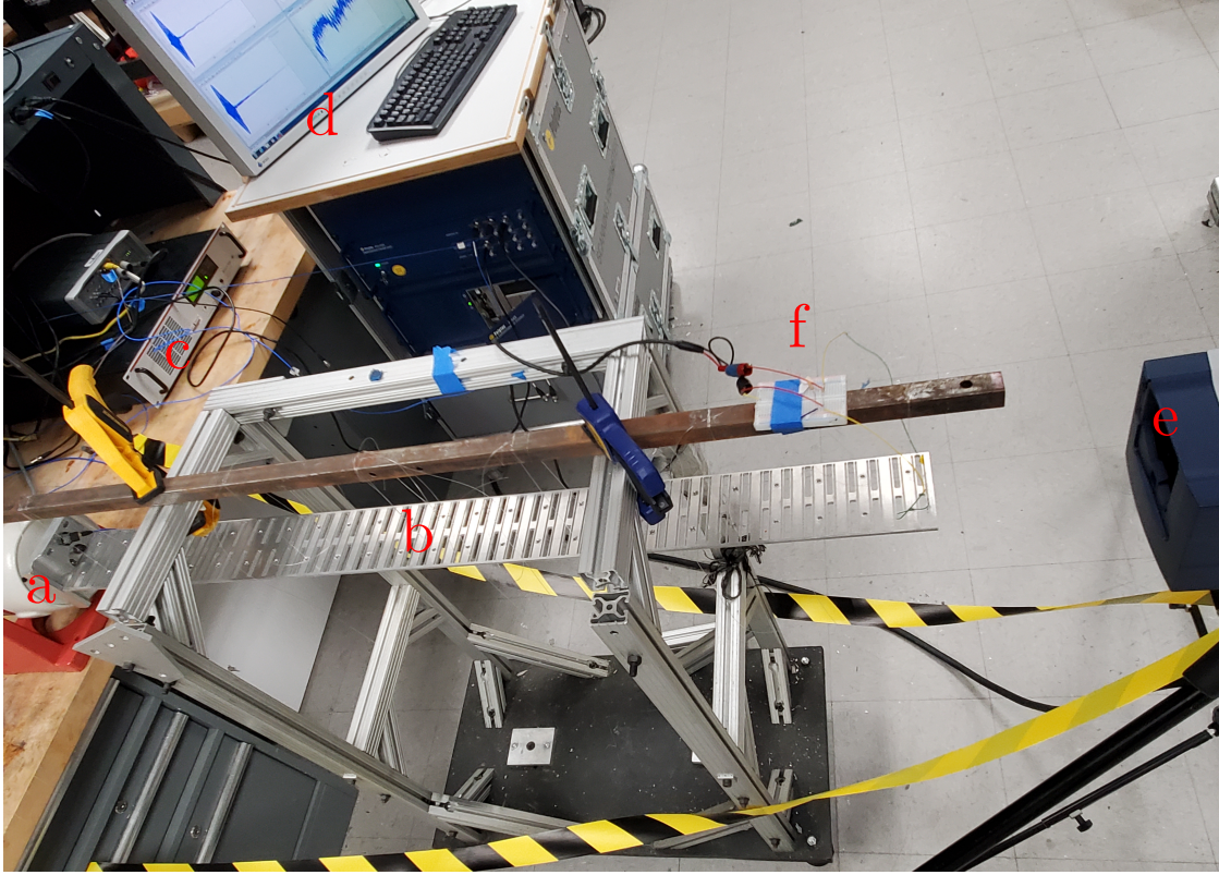
Figure 5.16: Experimental setup of the metastructure prototype: (a) Shaker, (b) prototype, (c) amplifier, (d) analyzer, (e) laser doppler, (f) shunted circuit.
