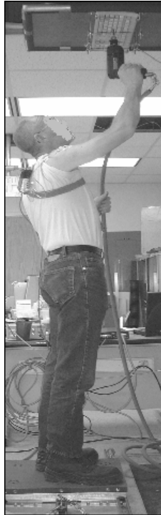
Figure 4.4 Participant shown performing the overhead task using drill tool.
